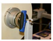
The mandrel has a hinged support and provides a handy storage for the T-bar Allen key.
