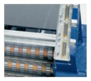
When inserting the automatic fold plates into the fold unit, electrical connection is achieved automatically, no more tangled cables and plugs.
