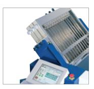
All fold plates feature automatic setting. This means that setting measurements can be entered by touch-screen, with a precision of 0.1 mm. Moreover, corrections are possible while the machine is running. The length of the fold plates is the same in all fold units. Therefore, no errors will occur when fold plates are inserted in different positions.
