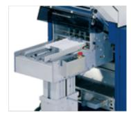
Small format vertical stacker SKM 36 especially for small folds.
