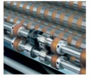
Easily accessible delivery shafts for scoring, perforating and cutting tools.
