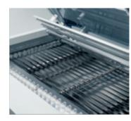
Register table with antistatic lattice-type surface.
