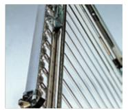
Deflectors have an important function. Consequently they have been designed so that their uninterrupted surfaces make for smooth paper travel and eliminate nicks and marks
