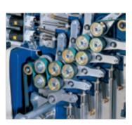
Fold rollers are driven from both sides by maintenance-free belts, resulting in perfectly synchronized operation.
