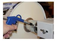
The film mandrel swings out and has an air shaft to speed roll changes.
