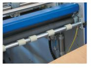
The adjustable burster automatically separates sheets up to B2 size.
