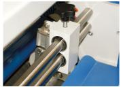
The positioning of the pneumatically controlled perforator overcomes any potential issues caused by poor film roll profiles and allows higher speeds to be maintained.
