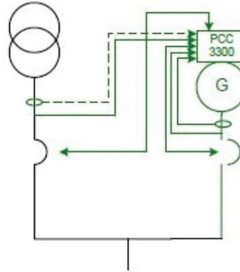
**Utility single:** Control monitors one genset and utility. The control will automatically start and provide power to a load if the utility fails. The control will also resynchronize the genset back to the utility and provides extended paralleling capabilities.
