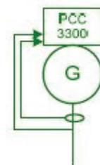
Synchronizer only: control will synchronize the genset to other source when commanded to either via a hardwired or Modbus driven input.
