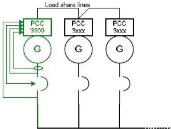
**Power transfer control:** control operates a single genset/single utility transfer pair in open transition, fast closed transition, or soft closed transition. Extended paralleling functionality also provides base load and peak shave options.
