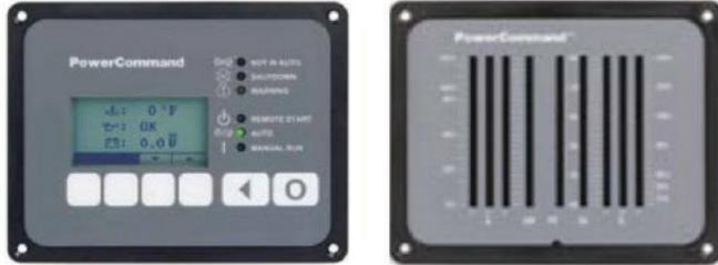
**PowerCommand control** is an integrated generator set control system providing voltage regulation, engine protection, operator interface and isochronous governing (optional). Major features include:
