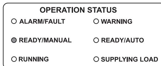
3. The LCD window will indicate “MAN” (manual) mode and “Ready.” The Ready/Manual LED will be lit. **Note:** The unit must be in the “MAN” Mode with the Ready/Manual LED lit to start the unit.
