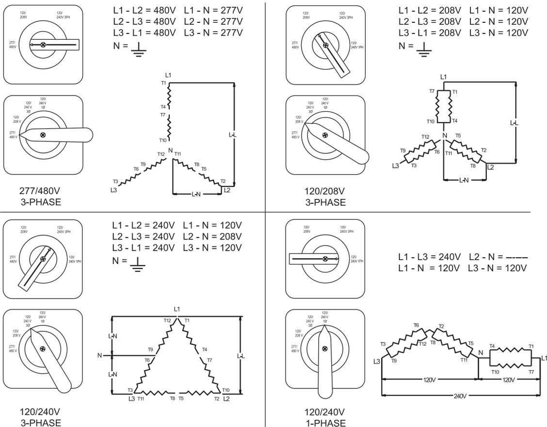
The voltage selector switch is equipped with a locking mechanism. Once the proper voltage has been selected, push the red latch on the inside of the switch handle up and insert a padlock through the handle. By locking the handle in place you will prevent unauthorized personnel from changing the switch settings.
