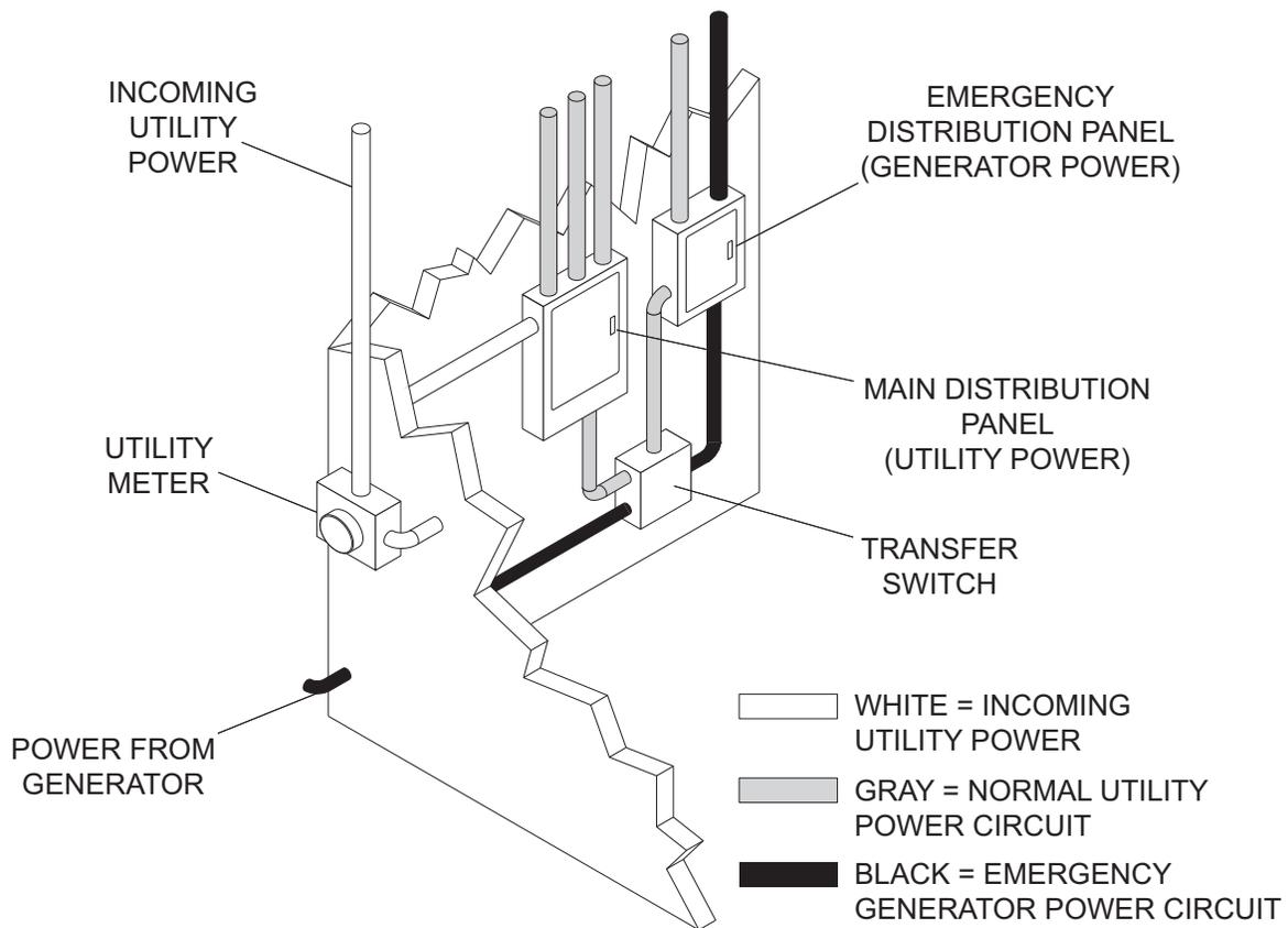
Installation of a transfer switch or other type of remote starting device is the responsibility of the generator user. Installation of such devices must be performed by following all directions supplied by the manufacturer of the switch. If attaching the generator to a power supply normally serviced by a utility company, notify the utility company and check local and state regulations. Familiarize yourself with all instructions and warning labels supplied with the switch.
