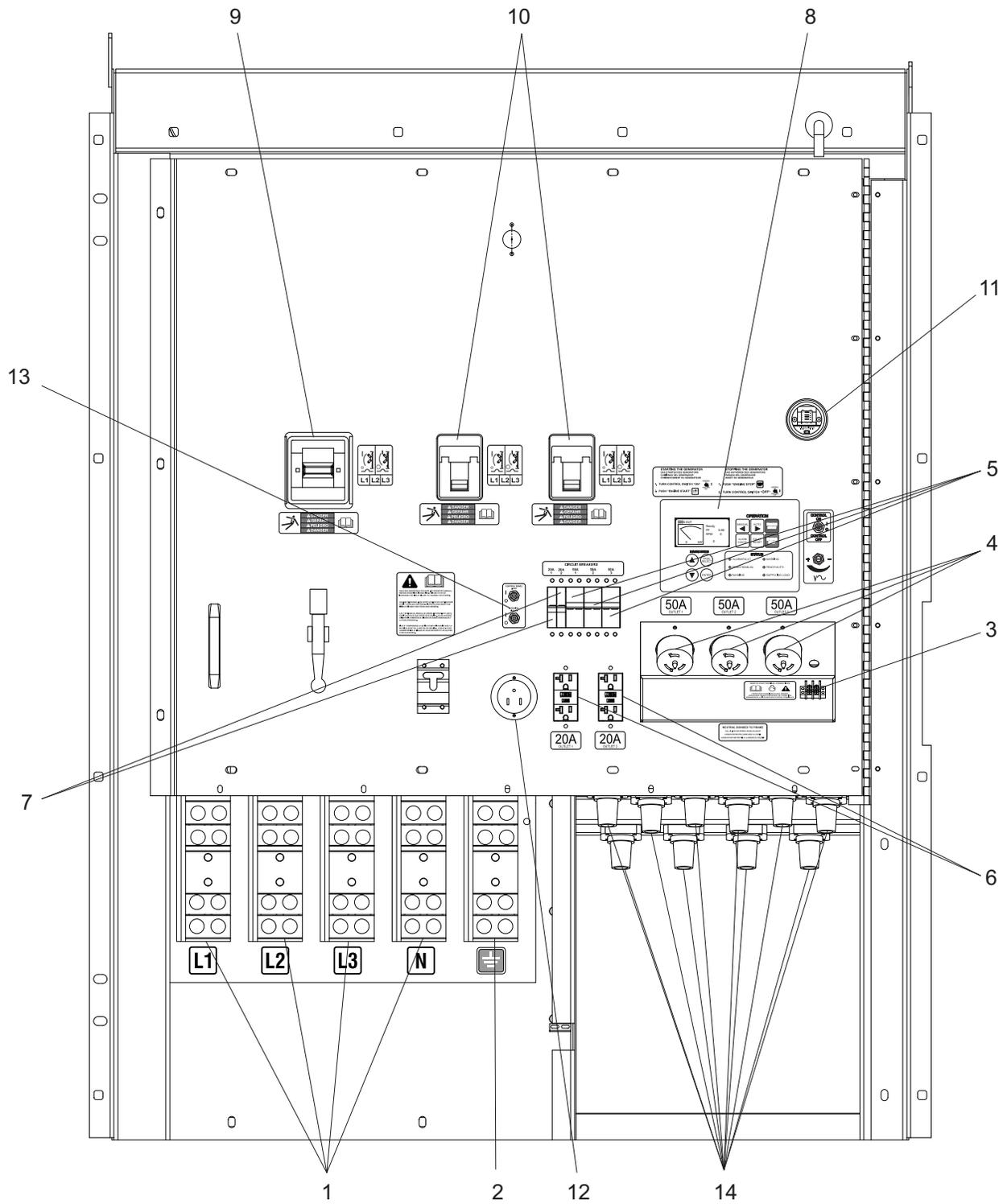
1. **CONNECTION TERMINAL LUGS:** External loads are wired to these lugs.
