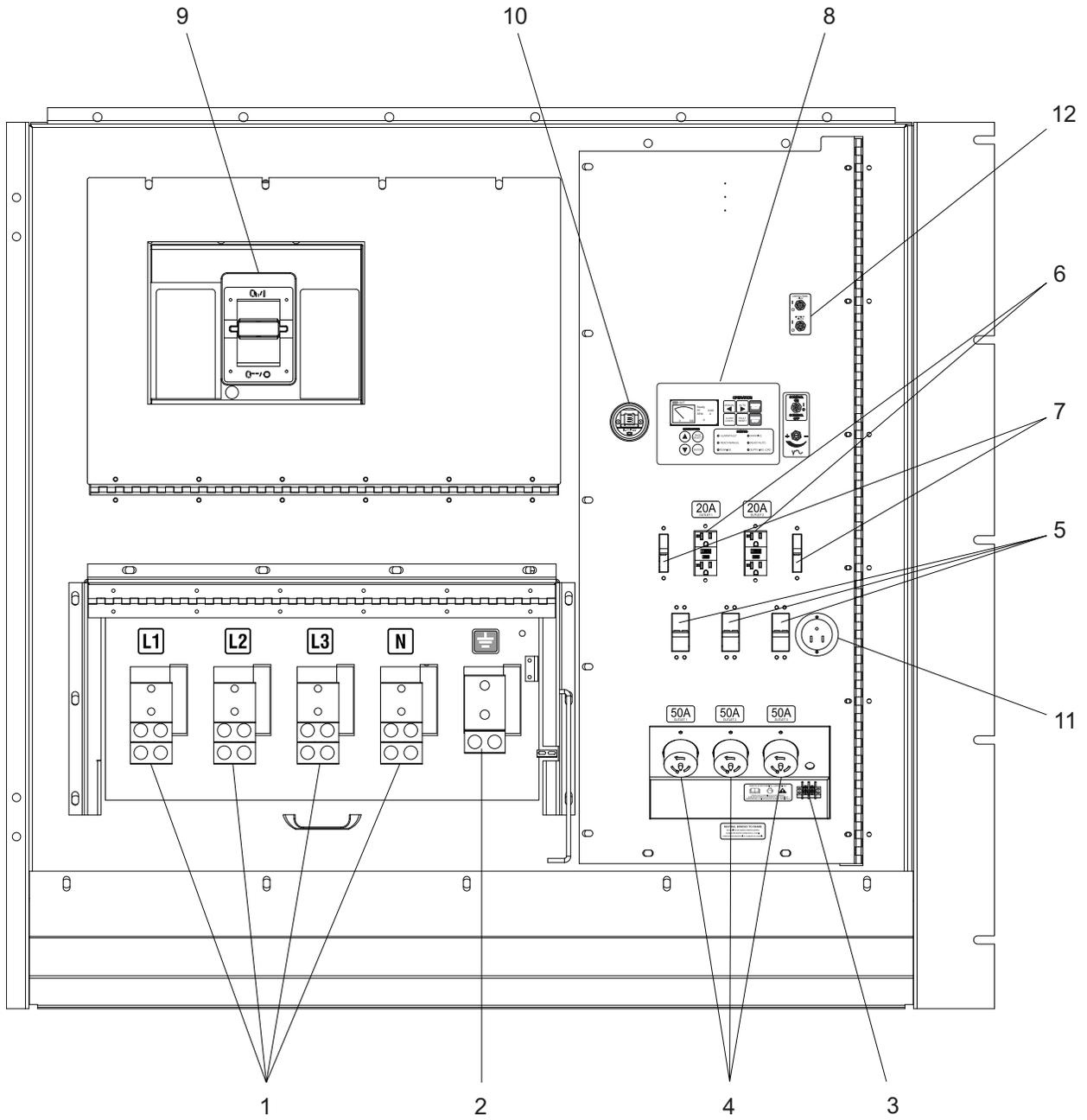
1. **CONNECTION TERMINAL LUGS:** External loads are wired to these lugs.
