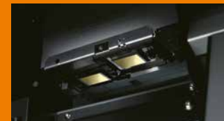
Dual print heads in staggered formation.
