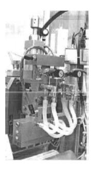
A continuous flow of water allows to avoid overheating of the groups.
