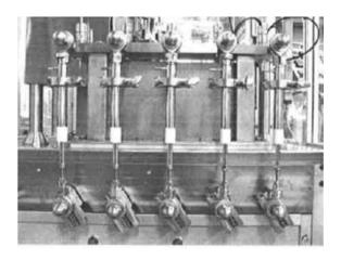
The movement that determines the dosage is controlled by a dedicated brushless motor. A potentiometer is installed on the control panel which allows the machine speed to be adjusted according to the product to be dosed.
