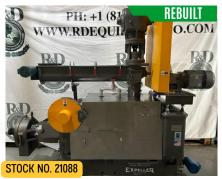
Rebuilt Expeller Press configured to extract oil from desiccated coconut to make VCO
