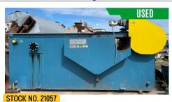
Reduces the sediments from the oil, before the oil its sent to a pressure leaf filter for further filtration.
