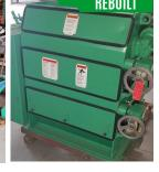
Cracks grains and oilseeds into smaller uniform particles prior to processing.
