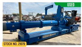
Mechanically shears, cooks and dries the material being processed for improved oil recovery coming from an expeller press.
