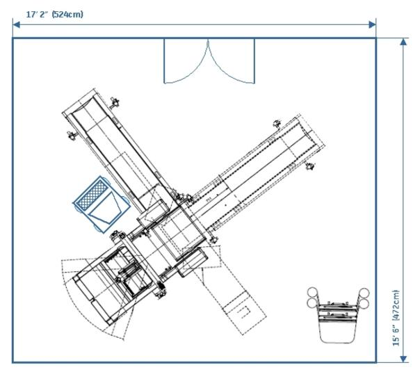
The above drawing meets clearance requirements under U.S. Federal Regulations and National Standards: 29 CFR 1910 (OSHA), NFPA 70E (Standard for Electrical Safety in the Workspace), and NFPA 101 (Life Safety Code). Specific room layouts are also subject to local and regulatory requirements.
