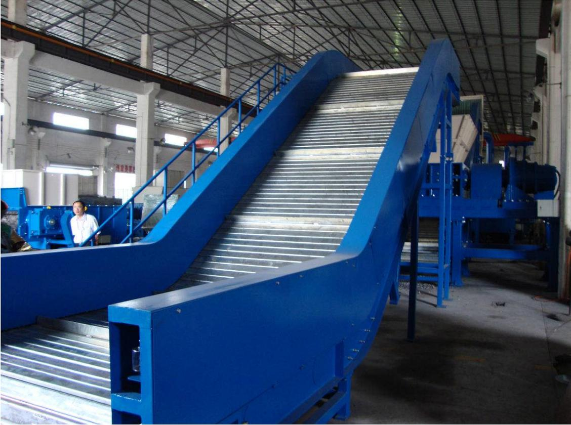
**This is a picture of infeed and discharge conveyors that are used in the system. Although there are three conveyors in the picture the system uses two of these conveyors for the infeed of material into the primary shredder and for the discharge and infeed of material into the secondary shredder.**
