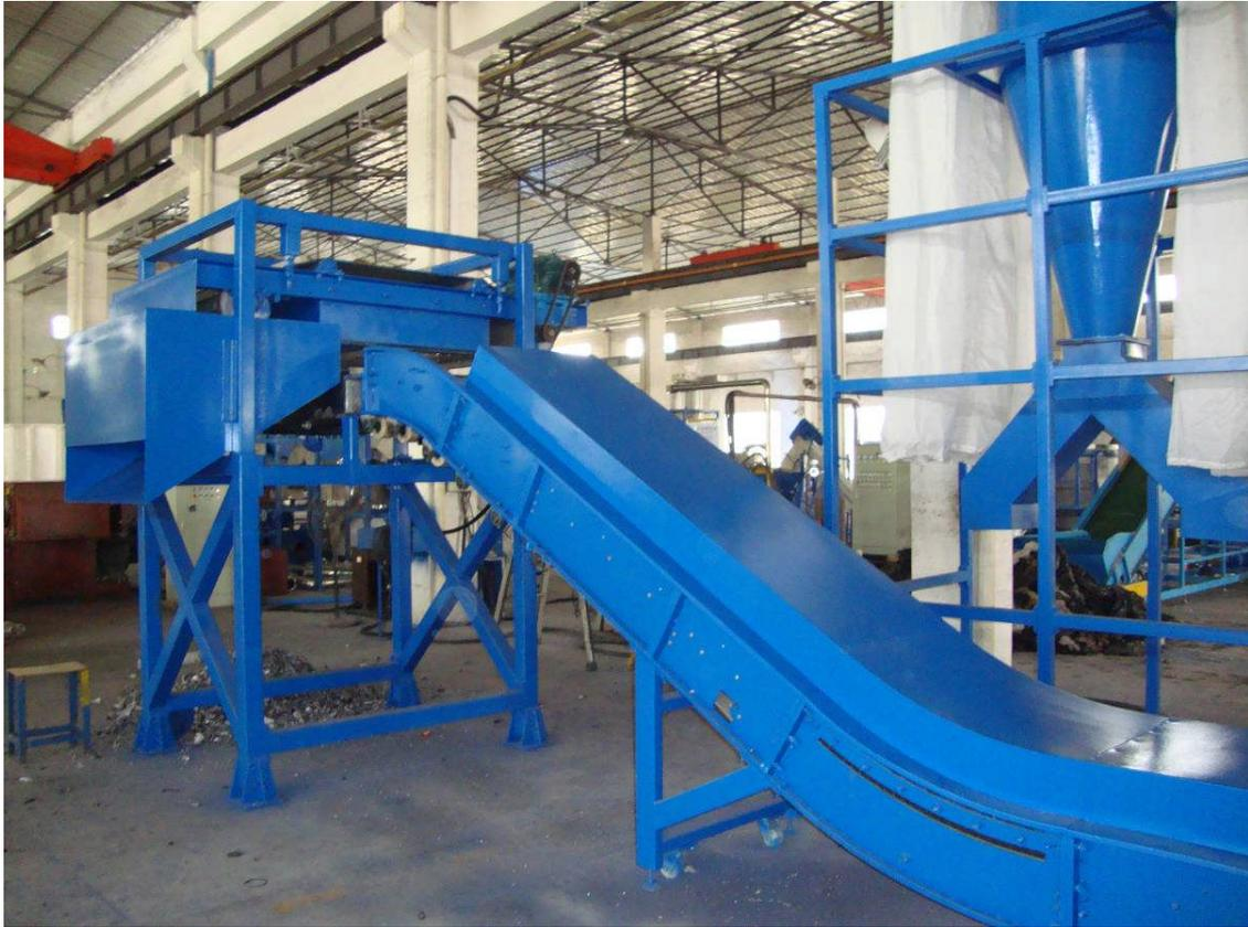
**The two shredder system ( 7272-V400 ) design is one of our standard shredding system packages. We can design shredders and shredding systems to suit almost any budget. The three shredder system ( 7272, 7272, V400 is suited to make higher volumes of product through the system.**
