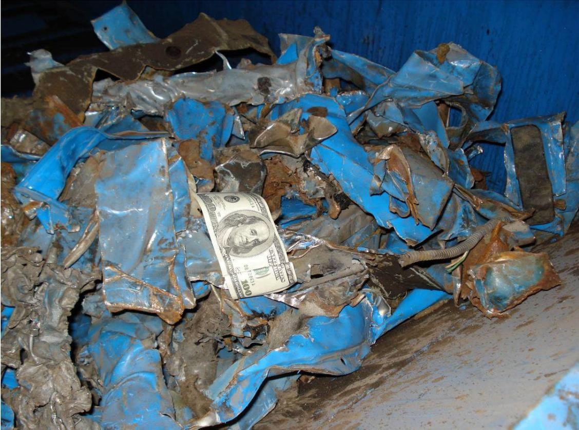
**This is the actual size of the primary shredder metal scrap which is set on a 3" wide cut to produce a strip of shredded stock that can be fed into the vertical grinder for final processing into a dense 80 pound per cubic foot frag for optimum value to you as a shredder company.**
