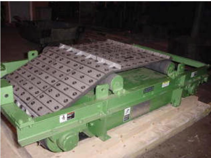
**This is a picture of the type of magnet that is provided in our system that removes the ferrous frag from the discharge conveyor in the system.**
