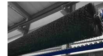
Brush cleaning springs
