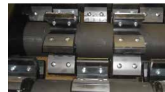
Wear plates on polyurethane screening stars
