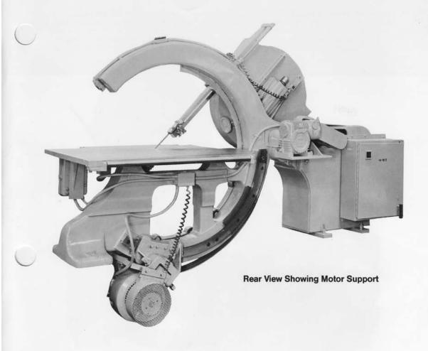
**Controls** are of the magnetic type grouped in a control box at the rear of the machine, the angling motor is provided with a reversing switch. A centralized push button control panel is mounted on the front of the table and provides the following controls:
