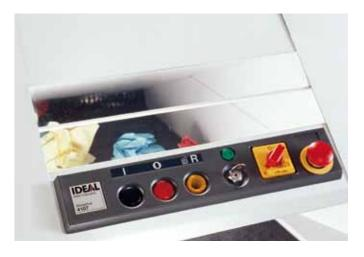
**CONTROL PANEL** Ergonomically placed control panel with push buttons for forward / stop / reverse and optical indicators for the operational status of the shredder.
