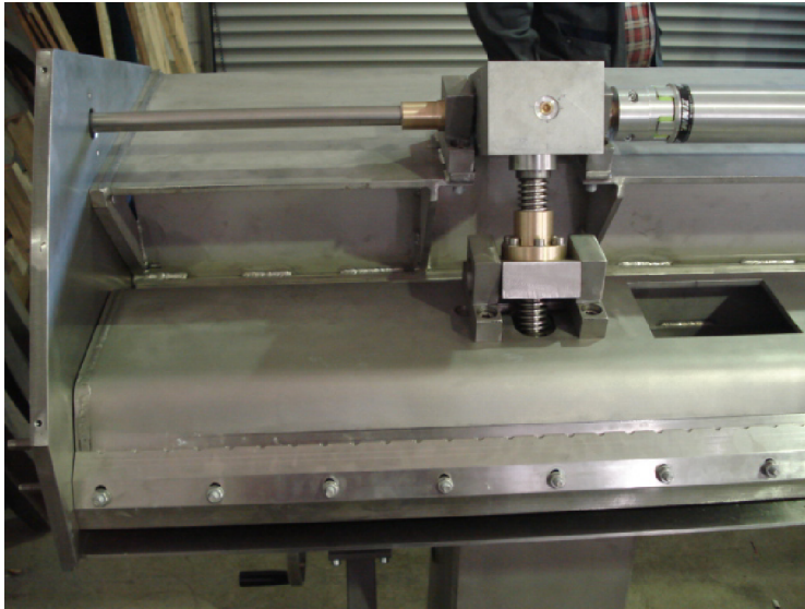
Tending Side Gearbox w/ Extension shaft to Handwheel
