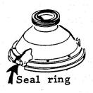
Place bowl parts on a soft base, such as wood or rubber. Be special careful of the seal ring in the lower edge of the bowl hood.
