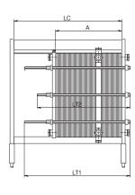
The overall length (LC) as well as A, LT1 and LT2 vary, depending on the number of plates and connection plates. The recommended free space along the sides of the unit and at the front end is 1.5 m.
