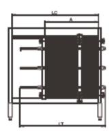
The overall length (LC) as well as A and LT vary, depending on the number of plates and connection plates. The recommended free space along the sides of the unit and at the front end is 1.5 m.
