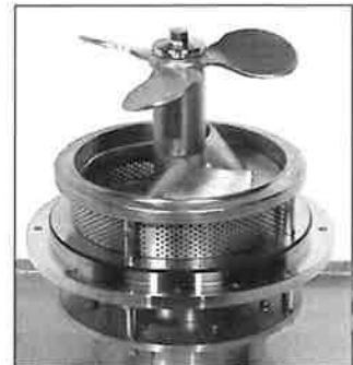
The stator in lowered position. High shear mixing.
