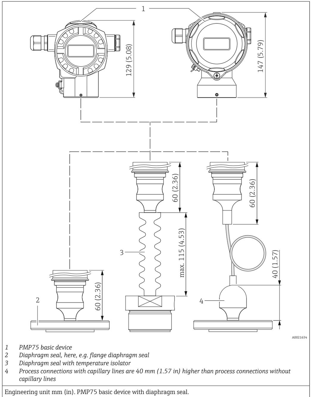
Process connections PMP75, flush process membrane
