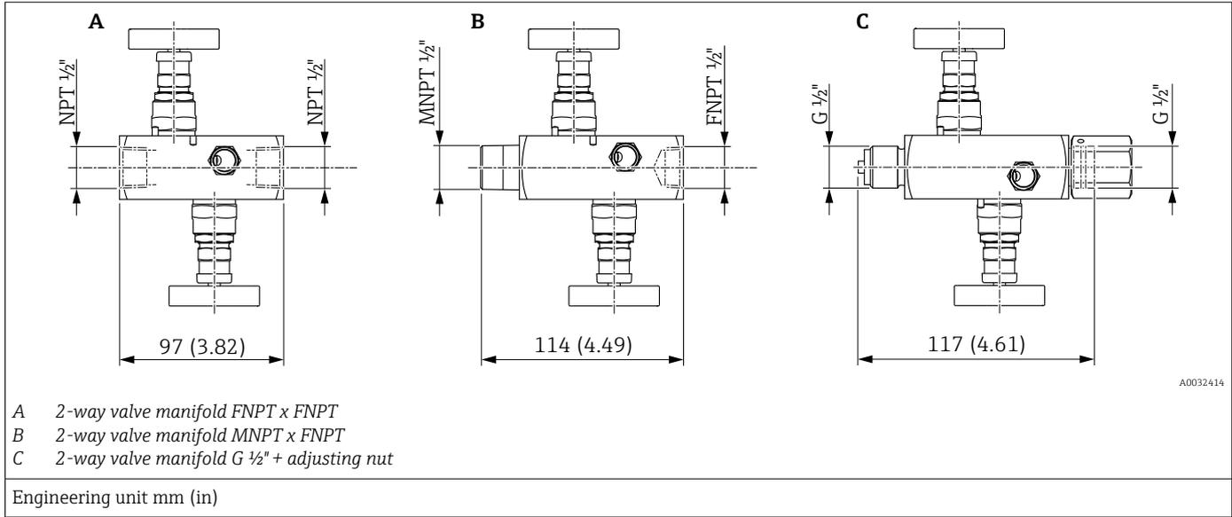
2-way valve manifolds in 316L or AlloyC can be
