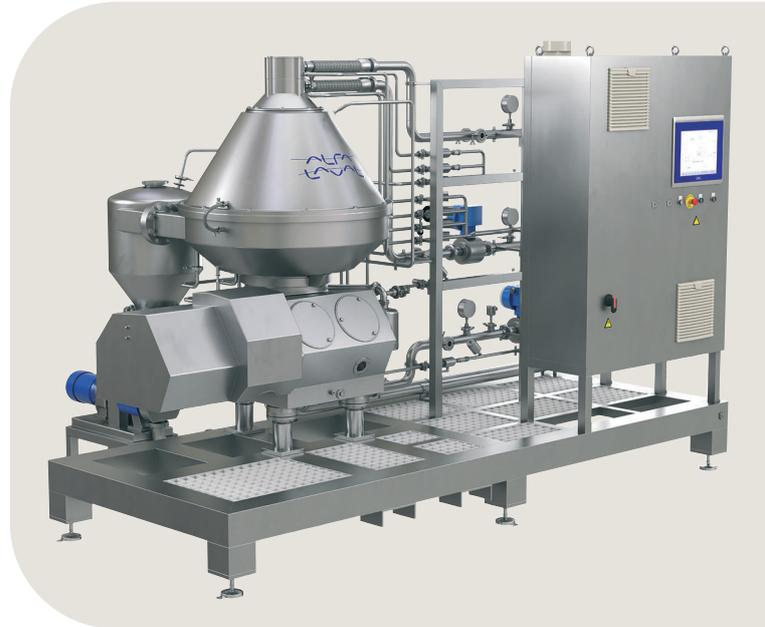
All metallic parts in connection with the process liquid are made of stainless steel.
