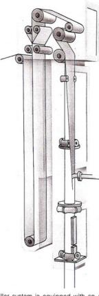
The filler system is equipped with an AP (Aseptic Product) valve. This makes it possible to wash the filler system of the machine while the product is still in the product conduit connected to the machine.
