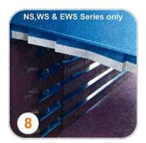
Single cylinder bale tensioning system with linkage bars provides up to 1 million pounds of extrusion force!
