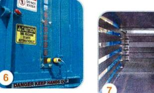
The in-feed hopper has a gasketed access door and viewing windows on both sides of the hopper. Infrareds are adjustable the entire height of the hopper door window.
