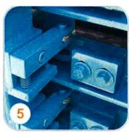
Wire positioners on twister cabinet side for precise twister alignment and no missed wire pick-ups.
