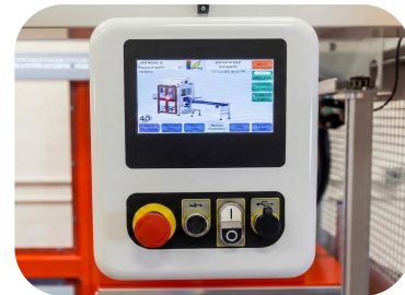
7" HMI touchscreen with Panel PC controls Quick changeover with 50-recipe memory
