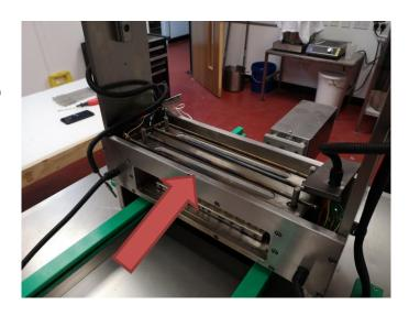
10. To remove the nozzle plate, lift the plate upwards and outwards.
