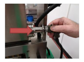
3. Unscrew and remove the oil tank thermostat.
