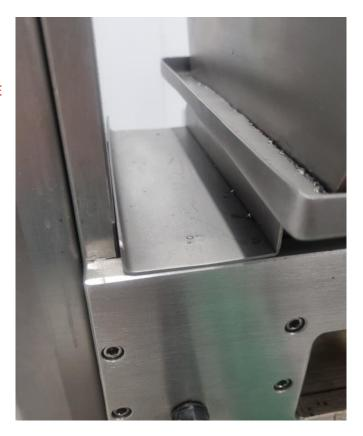
9. Image showing the hopper removed and the heating elements exposed.
