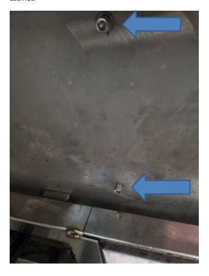
Once these have been removed the green mould track can be removed to expose the bolts retaining the bottom heaters.
