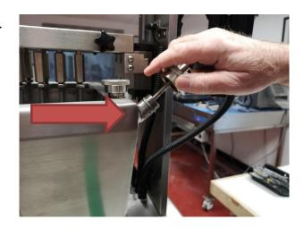
4. Unscrew the piston retaining knob.
