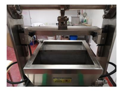
7. Now all the pistons have been removed you can continue to remove the hopper from the machine.
