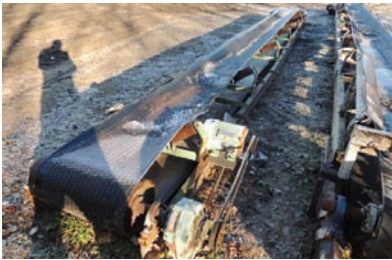
9139 $7,500.00 BELT CONVEYOR concave belt conveyor, 24" wide x 30' long, electric drive, good condition 260-633-4047
