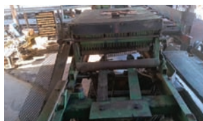
Edmiston's Edger Serial #: HE30-4. Model: 30-4. Features and Notes: 4"x30", 2 movable saws, hydraulic controls, no power-belt drive, belt outfield table.
