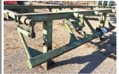
9244 $8,000.00 CANT CATCHER Reckart cant catcher for drop use with a drop belt, air powered, 4 arms, travel is 30", good working condition 260-633-4047
