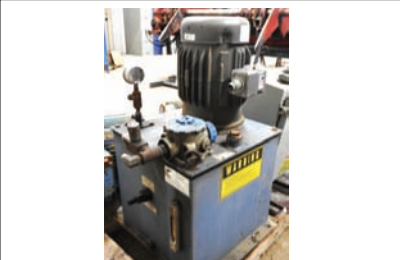
18241 $1,250.00 HYD UNIT Continental hyd power unit, 5 hp electric drive, pressure comp pump, approx 10 gal reservoir, good working condition 260-633-4047
