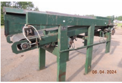
9191 DROP BELT $9,500.00 Pendul slab drop belt, 24" wide x 10' 6" long, hyd drive, twin air cylinders for up-down on belt, heavy duty and in excellent condition 260-633-4047
