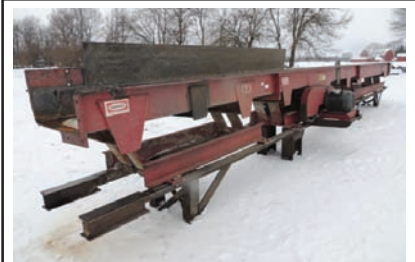
9126 VIBRATING CONVEYOR $21,000.00 Mellott 24" wide pan x 62' long, sawdust screen section, 8" tall sides, electric drive, good working condition 260-633-4047
