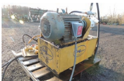
18236 $1,750.00 HYD UNIT 10 hp electric powered, vane type pump, approx 25 gal capacity, includes several flow ctrls, excellent condition 260-633-4047
