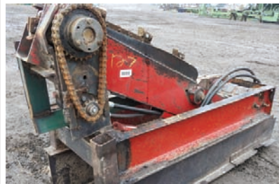
8059 $4,200.00 LOG TURNER chain type log turner, 36" chain, hyd drive, good working condition 260-633-4047
