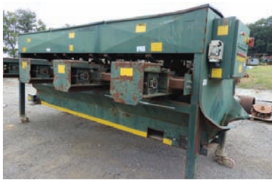
17114 $27,500.00 TRIM SAW 4 head trim saw, up to 12' long capacity, electric powered, includes material and waste belts, price includes going through shop, ready for production 260-633-4047
