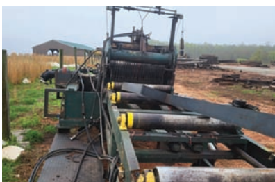
5126 $17,250.00 EDGER Cooks edger, 6" thick x 36" wide capacity, 2 movable blades, set up for tailing belt, hyd drive, includes controls, tailing belt, dust auger under edger, nice condition and ready for production 260-633-4047
