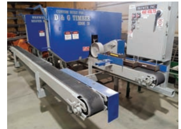
3601 $25,000.00 BREWER 2 HEAD RESAW 3 ph. 480v electrical powered, 30" band wheels, air strain, return belt. This is a reconditioned unit. Unit is 7' wide x 13' 9" long. Plug in ready. 260-740-8036
