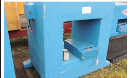
20270 METAL DETECTOR $6,000.00 MDI whole log metal detector, capacity is 30" wide x 28" tall, includes controls, very good condition 260-633-4047
