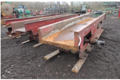
9236 $10,500.00 VIBRATING CONVEYOR 30' L, hyd drive, 24" pan, 8" sides, 19" from floor to bottom of pan, good condition 260-633-4047
