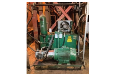
18240 $4,500.00 HYD POWER UNIT 40 hp electric drive hyd unit, pressure comp pump, includes cooling radiator and accumulator, very good condition 260-633-4047
