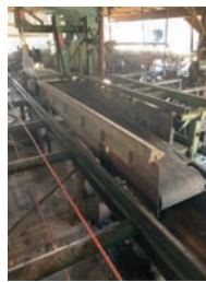
9243 $7,200.00 DROP BELT CONVEYOR Reckart drop belt, 24" wide x 13' long, air cylinder for up-down, hyd drive, good working condition 260-633-4047
