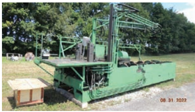
6031 HMC DEBARKER $34,500.00 rosser head style, all hyd. drive, 36" dia. log capacity x 12' long, very good condition 260-633-4047
