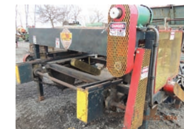
17103 TRIM SAW $8,500.00 Morgan double end trim saw, Serial # 062800311, minimum 20", max. 60" wide capacity, electric drive, very good condition 260-633-4047
