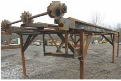
9260 $1,850.00 TRANSFER DECK transfer/ log deck, 3 strands, 8' wide x 20' long, H-78 chains, working condition 260-633-4047
