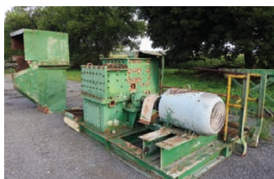
7155 $8,500.00 WASTE GRINDER Progress waste grinder, swinging hammer style, 125 hp electric drive, 1185 rpm's, unit needs to have hammers installed, good overall condition 260-633-4047
