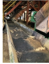
9256 VIBRATING CONVEYOR $28,750.00 Webster vibrating conveyor, 24" wide pan 9" tall sides, 80' long, electric drive, very good condition 260-633-4047
