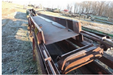
9141 $7,500.00 BELT CONVEYOR 24" wide x 68' long belt conveyor, approx 6" tall sides, electric drive, good condition 260-633-4047
