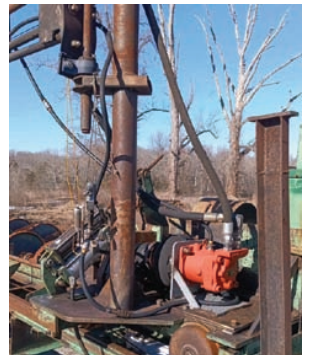
HMC Debarker Serial #: unknown. Model: slant track . Features and Notes: Slant track, Bark King head, hydraulic drive, uninstalled but was in production up until removed
