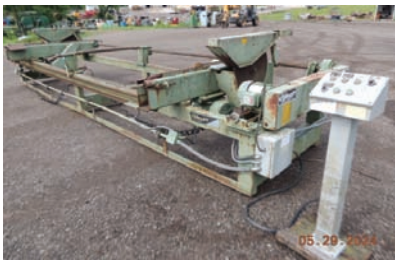
17108 $9,500.00 DOUBLE END TRIMMER Corley double end trim saw, 8" thick capacity, electric drive, good working condition 260-633-4047
