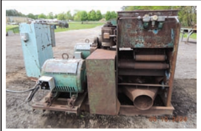
4037 GANG SAW $9,500.00 Cornell double arbor gang saw, 6" thick x 24" wide capacity, 2- 100 hp electric motors for arbors, working condition 260-633-4047
