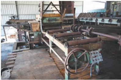
5114 $10,750.00 COOK EDGER Model:36EZTD, SN: 42, 5" x 21' tailing belt outfeed, 38" x 9' infeed rolls, 6" x 36" infeed cap, control panel, manual blade set, (2) 20" blades both are adjustable, electric drive, good heavy duty older unit 260-633-4047
