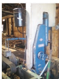
1608 $16,000.00 VERTICAL 3" BAND HEAD 30" wheels, top guide is hand crank, 32" opening, has weight strain and is in working condition. 724-967-3318
