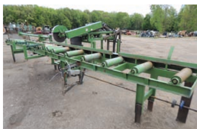
17104 CHOPSAW $12,500.00 chop saw for cants, 7" thick x 12 "wide capacity, 18" wide x 14' long infeed, 18" wide x 10' long out feed, 2 air powered stops, cant pusher arms, shop built, line-shaft and air operated, good working condition 260-633-4047
