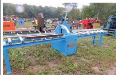
17094 PROCUT CHOP SAW $9,079.00 up-cut style, 7" x9" cutting capacity, 22" dia blade, includes 8' infeed/outfeed, 4 flip stops, BRAND NEW, buy this one or order one to your specs 260-633-4047
