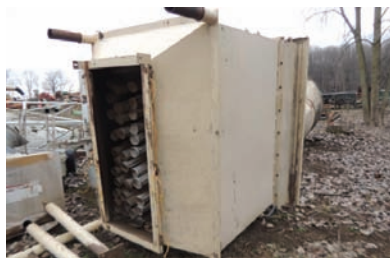
10309 $4,000.00 BAG HOUSE SYSTEM Honeyville Metal baghouse is approx. 8' x 8', 72 - 5" x 60" bags, 11" x 13" inlet, 28" x 63" bottom outlet, includes blower and numerous pipes, good condition 260-633-4047
