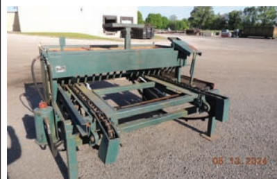
17105 DOUBLE END TRIM SAW $8,500.00 Morgan double end trim saw, 6" thick x 68" long capacity, line-shaft ready, feed is hyd driven, good operating condition 260-633-4047
