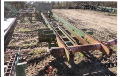
9096 TRANSFER DECK $4,250.00 2 strand transfer deck, 3' wide x 25' long, electric drive, 81X chain, good condition 260-633-4047
