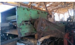
Edmiston's Edger Serial #: HE30-4. Model: 30-4. Features and Notes: 4"x30", 2 movable saws, hydraulic controls, no power-belt drive, belt outfield table.
