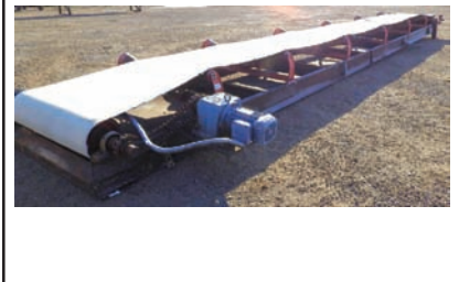
9219 CONCAVE BELT CONVEYOR $7,000.00 36" wide x 30' long, electric gear box drive, good working condition 260-633-4047
