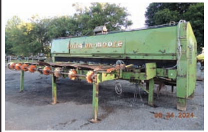
17112 $17,500.00 TRIMMER drop trimmer, 9 blades, up to 18' long capacity, air cylinders on heads, electric powered, price does not include going through shop 260-633-4047
