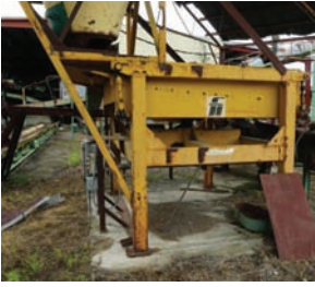
7093 $11,500.00 FULGHUM SHAKER SCREEN 8' x 8' screen, electric drive, includes the chip cyclone, good condition 260-633-4047
