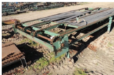
9249 $5,000.00 TRANSFER DECK 4 strand, 10' wide x 22' long, H-78 chain, good condition 260-633-4047
