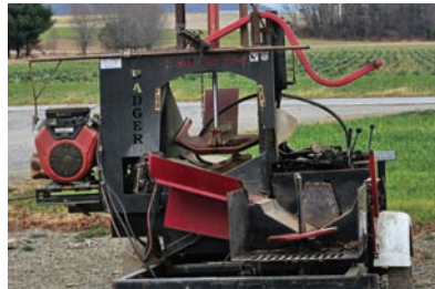
20610 BADGER 4 WAY SPLITTER $10,000.00 Manually operated cutting bar, 20" x 24' in length capacity. 16 hp. on the saw and a 16 hp. on the hydraulic (gas motors). Put the log on the belt to bring it to the saw. Smoker Sawmill: 81 Utt Rd. Orangeville, PA, 17859 908-930-8820
