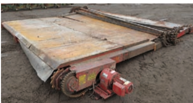
9220 SLAB DRAG DECK $8,500.00 slab drag, 15' x 15', electric gearbox drive, 81X chain with steel cleats bolted on, good working condition 260-633-4047
