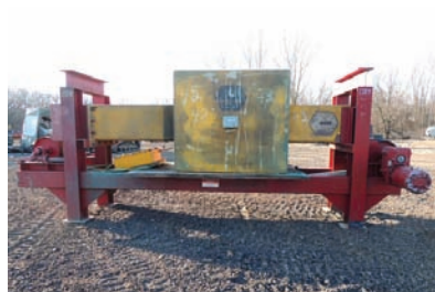
20274 METAL DETECTOR $11,500.00 18"W belt 22" opening 15' long 74" high, excellent condition 260-633-4047
