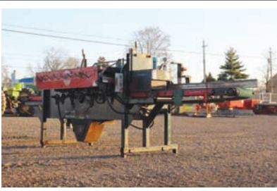
4035 GANG SAW $17,250.00 Morgan single arbor gang saw, capacity 12" wide x 5 1/2" thick, 100 hp electric drive on arbor, feed rolls are hyd drive, includes spare spacers, could be used for scragg slab edger, good condition and ready to work 260-633-4047
