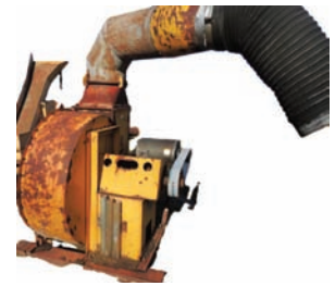
10349 DUST BLOWER 48" dia blower, 17" inlet/ 16" outlet, 40 hp electric power, good condition 260-633-4047
