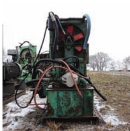
18191 CARRIAGE DRIVE $2,850.00 75hp electric, double pilot pump, directional valve 260-633-4047
