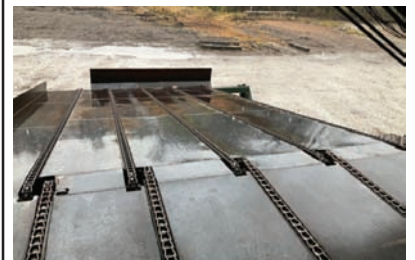
9253 $8,500.00 TRANSFER DECK 5 strand heavy duty deck, 12' 6" wide x 25' long, electric drive, H-78 chain, very good condition 260-633-4047
