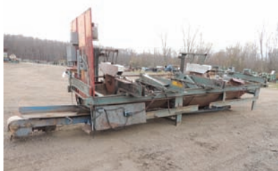
17079 TRIM SAW $5,750.00 double end trim, 22" blades, electric drive, 16' long capacity, good condition 260-633-4047
