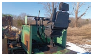
HMC Debarker Serial #: unknown. Model: slant track . Features and Notes: Slant track, Bark King head, hydraulic drive, uninstalled but was in production up until removed
