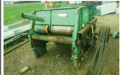
5089 SHURMAN GANG EDGER $17,250.00 6"x42" wide overall, includes infeed and outfeed rollers, working condition 260-633-4047
