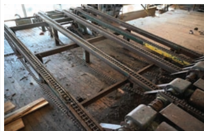
9018 $4,600.00 TRANSFER DECK 5 strand, 13' wide x 18' 6" long, H78 chain, electric drive, air cylinders on pop up board stop, good condition 260-633-4047
