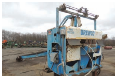
5122 $13,500.00 BREWCO EDGER 4" thick x 20" wide capacity, powered by 2 separate electric motors, includes 16' long tailing belt, unit is in very good working condition 260-633-4047
