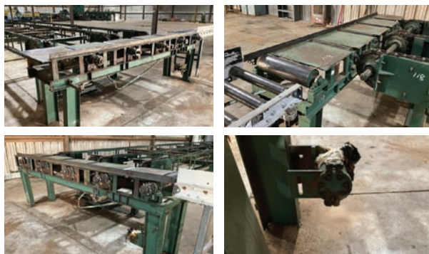
Live Rollcase Drive Type: None. Overall Dimensions: 28" x 10'. Roller Size: 5" x 18". Shaft Size: 1 1/2". Features and Notes: Not fully set up, no drive chains.
