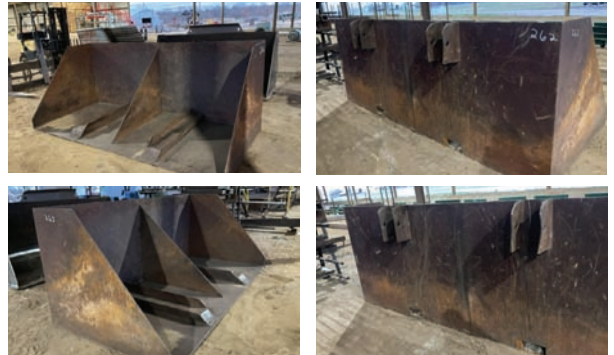
Dust Bucket 10' x 54" x 46", slip on bucket built with 1/2" steel.
