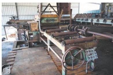
5114 COOK EDGER $10,750.00 Model:36EZTD, SN: 42, 5" x 21' tailing belt outfeed, 38" x 9' infeed rolls, 6" x 36" infeed cap, control panel, manual blade set, (2) 20" blades both are adjustable, electric drive, good heavy duty older unit 260-633-4047
