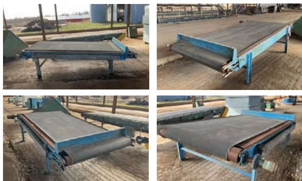
Belt Conveyor Length: 10'. Belt Width: 54". Drive Type: Hydraulic. Overall Width: 62". Features and Notes: Was bought for edger outfeed.
