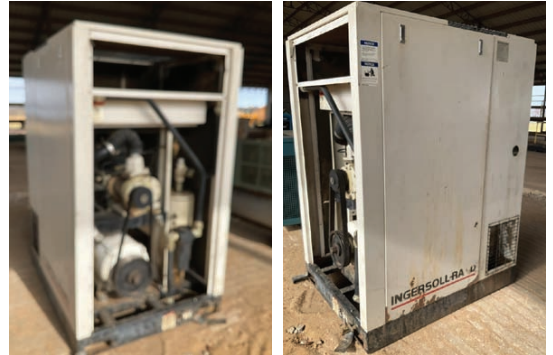
Ingersoll Rand Screw Type Air Compressor Model SSR-EP50SE, SN: G55O8U97010, 50 hp electric motor, belt driven compressor, bad motor all else is good.
