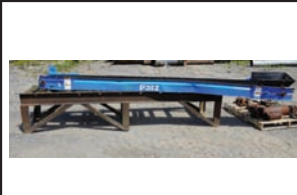
Patz Belt Conveyor and Rollcase 12" x 12' 4" conveyor, 12" belt, no power, 31" x 10' dead rolls, 3 1/2" x 26" rolls
