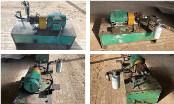
Hydraulic Pack 10 hp electric motor on pump, 4' x 2' x 1' tank.
