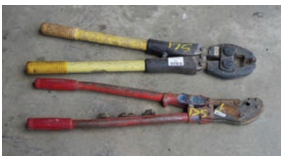
Kearney Crimp Tool (2) Heavy wire crimp tools
