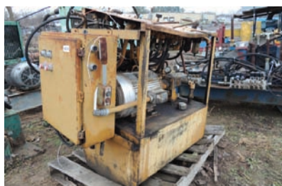
18210 HYD UNIT $2,000.00 used on Fulghum rosser-head debarker, 15 hp electric drive, 2 stage vane type pump, approx 45 gal tank, working condition 260-633-4047
