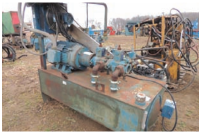
18186 HYDRAULIC PACK $5,000.00 30 HP electric motor w/double pump direct mouter, approx. 100 gal tank, lots of electric control valves, oil cooler, electric control box 260-633-4047
