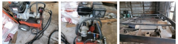
Shop-Built Mat Drilling Machine Shop built mat drilling machine powered by a portable hydraulic unit with a 13 hp gas engine. 8' x 15' x 41 1/2" drilling bed, 3 Ply mat unit, hydraulic unit used only 7 months
