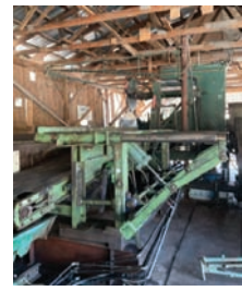
9244 CANT CATCHER $8,000.00 Reckart cant catcher for drop use with a drop belt, air powered, 4 arms, travel is 30", good working condition 260-633-4047
