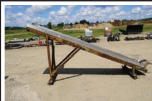
Belt Conveyor 22" x 12', no belt, stainless pan
