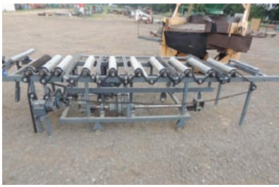
9080 $5,000.00 ROLL CASE/TRANSFER roll case with transfer, 26" wide x 11' long, 5 strand pop-up transfer, all mechanical and line shaft ready, like new condition 260-633-4047
