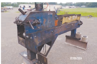
14076 $5,250.00 DUDUSTER Dyna model 80 deduster, 6" wide capacity, all hyd driven, new brushes included, good working condition 260-633-4047
