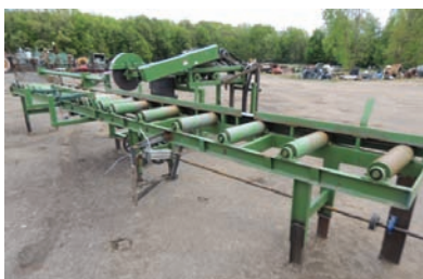
17104 CHOPSAW $12,500.00 chop saw for cants, 7" thick x 12 "wide capacity, 18" wide x 14' long infeed, 18" wide x 10' long out feed, 2 air powered stops, cant pusher arms, shop built, line-shaft and air operated, good working condition 260-633-4047
