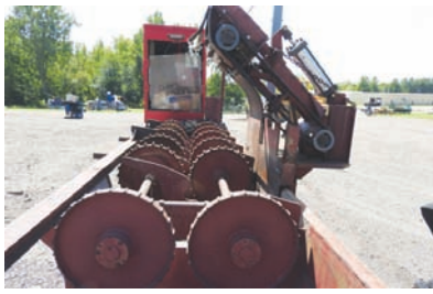
6046 DEBARKER $42,500.00 Mellott rosser-head debarker, your choice of power (electric or hyd), new babbitt in bearings, new cleats on bull wheels, good condition and ready for production 260-633-4047
