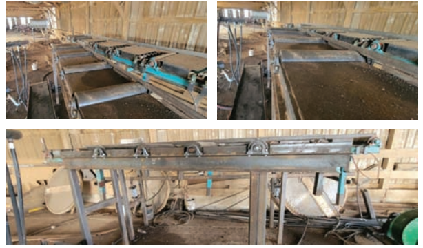
Shop-Built Rollcase Overall dimension: Unknown. Shaft Size: 1 3/8". Roller Size: 24" x 6". Drive type: None. Features & Notes: No drive. 24'x11'x78".
