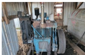
Quincy Air Compressor with Kubota Power Unit Fuel: Diesel. Features & Notes: 40 hp Kubota engine with 20 hp Quincy air compressor. Very good condition. Has automation control box.
