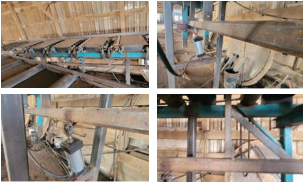
Rollcase with Transfer Overall Dimensions: 20' x 24". Shaft Size: 1 15/16". Roller Size: 24" x 8". With pop-up lumber dump.
