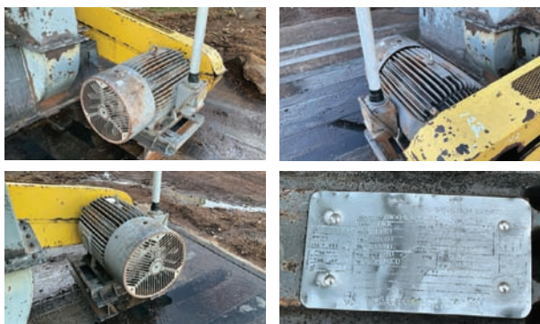
Toshiba Electric Motor Horsepower: 100. Frame Size: 405T. Phase: 3 Phase. RPM: 1765. Features and Notes: Includes wire and conduit to building .
