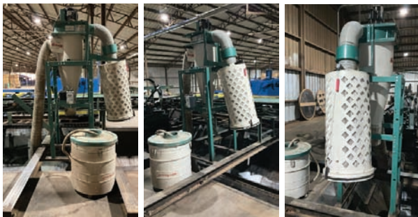
Grizzly Dust Blower Serial #: 150821. Model: GO441. Drive Type: Electric. Includes Pipe: yes. Inlet Size: 8". Outlet Size: 9". Size: 3 hp. Features and Notes: Blower on Top of cyclone, filter, collection barrel.
