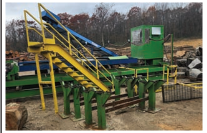
6601 PRECISION DEBARKER $32,000.00 Rebuilt in 2021 by Showcase Equipment. 50 Hp on the head & a 15 Hp on the hyd. electric motors. There is also an air compressor. 36" x 16' log capacity. You have the barn sweep, an extra head, legs steps catwalk included 814 594 9683
