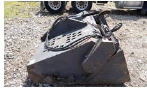
FFC Rockhound 76", hydraulic drive, skid steer quick attach
