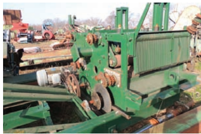
5103 TIERNEY GANG SAW/EDGER $85,000.00 6" capacity gang edger, gang side is 16" wide- edger side is 28" wide, this unit will be "SHOWCASE REBUILT" and come with a full warranty, call to customize to your specs and for a time-line 260-633-4047
