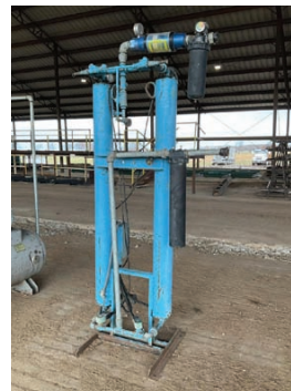
Air Dryer Twin tank air dryer, was working when taken out of production 2 years ago.
