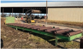
Rollcase Drive Type: None. Overall Dimensions: 75" x 36'. Roller Size: 6 1/2" x 48". Shaft Size: 1 5/8". Features and Notes: 55" x 35' dead rolls.
