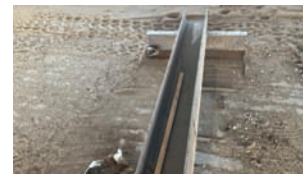
Pusher Arm 8" x 8" x 12' I- beam, slips on forks.
