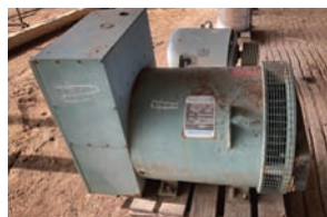
Generator Magna One, Synchronous AC generator, 1800 rpm, frame 500, 235 kw, model 500FDR8040GG-L282, condition unknown.
