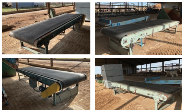
Hytrol Belt Conveyor Length: 12'. Belt Width: 36". Drive Type: Electric. Overall Width: 42".
