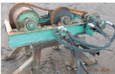
20308 CARRIAGE DRIVE $2,800.00 Helle cable drum unit for carriage drive, drum is 13 1/2" dia x 16" wide, hyd drive, good working condition 260-633-4047
