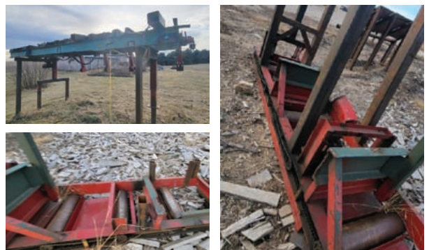
Mellot Transfer Deck & Rollcase Features & Notes: Transfer deck with hydraulic drive, 12"x6' with 2' pop up. 18"x12' roll case included. Good working assembly.
