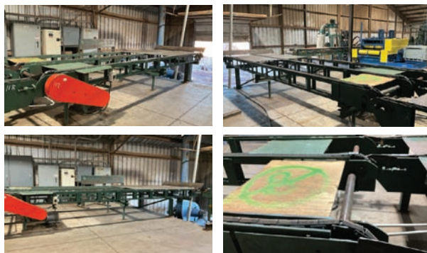
Greenchain Deck Model: na. Length: 22'. Width: 76". # of Strands: 3. Drive Type: Electric. Height: 40". Rooftop Chain: yes. Solid Decking: no. Features and Notes: 8' slant decking for side loading, side rail board stop.
