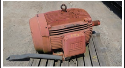
Weg Electric Motor 125 hp, 1780 RPM, 444T frame
