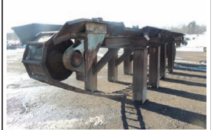
9090 $14,300.00 LOG TROUGH 40' long, 110 ladder-back chain, 14" wide, s-style drive, no power, good working condition 260-633-4047
