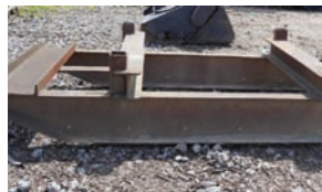
Steel Log Sled 62" x 12', post pockets
