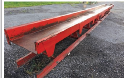
9207 VIBRATING CONVEYOR $11,500.00 Mellott vibrating conveyor, 24" wide pan, 8" tall sides, electric drive, chipper spout, very good condition 260-633-4047
