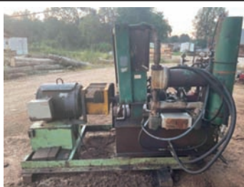
18166 $14,500.00 CARRIAGE DRIVE Tyrone SMA-270, 125hp electric drive, includes hyd unit and cable drum, good condition 260-633-4047
