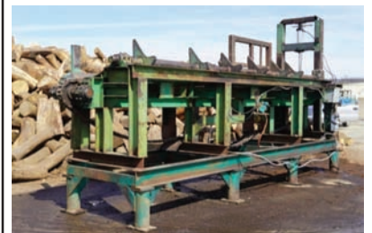
9238 $14,300.00 LOG TROUGH 50"x 22' overall, air cylinder log clamp down, electric drive, WR124 chain w/cleats, air cylinder on loader 260-633-4047
