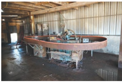
15078 $7,400.00 BAND SAW SHARPENER Armstrong, Model #6 RH, SN: 16154, electric drive, includes extra grinding wheels and all clamps and strands, Armstrong #58-B filling clamp, working condition 260-633-4047
