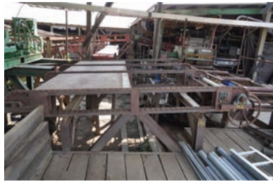
9227 $3,750.00 TRANSFER DECK 4 strand transfer deck, 10' 6" x 10' long, H-78 rooftop chain, electric gearbox drive, has board stops, good condition 260-633-4047
