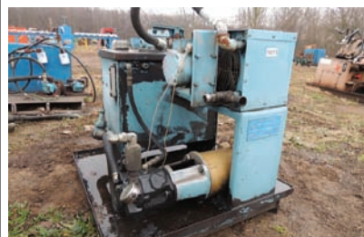
18213 HYD UNIT $2,000.00 5 hp electric drive, pressure comp pump, cooling radiator, approx 30 gal capacity tank, good condition 260-633-4047
