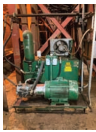
18240 HYD POWER UNIT $4,500.00 40 hp electric drive hyd unit, pressure comp pump, includes cooling radiator and accumulator, very good condition 260-633-4047
