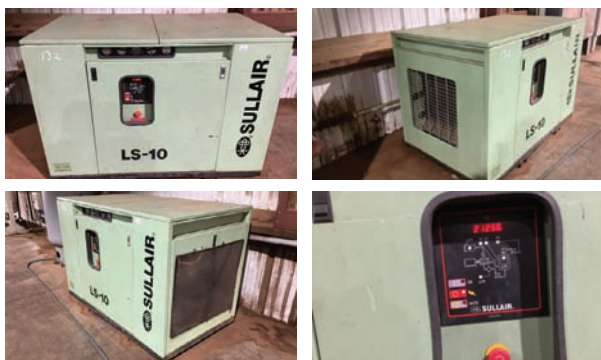
Sullair Air Compressor Model LS-10, meter reads 21256 hrs., screw type compressor, was being used on mill.
