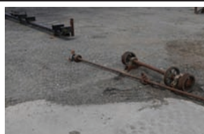
Lineshafts and Mounts 1 1/2" x 11' 6" shaft, 1 15/16" x 5' shaft, pulleys and bearings, 20' mounting beam
