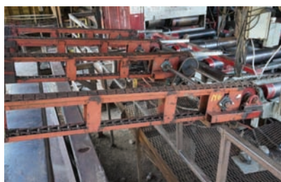
9222 TRANSFER DECK $3,750.00 4 strand transfer deck, 10' x 10', H-78 rooftop chain, hyd drive, air powered board stops, good condition 260-633-4047
