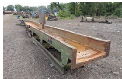
9066 $17,250.00 VIBRATING CONVEYOR Mellott 24" wide pan x 50' long, 8" sides, includes sawdust section and chipper mouth, hyd drive, good working condition 260-633-4047
