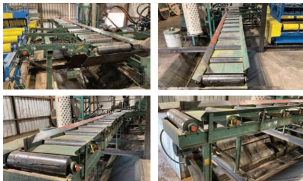
Rollcase with Side Transfer Drive Type: Electric. Overall Dimensions: 32" x 28' rollcase plus. Roll Type: Smooth Spiral. Roller Size: 61/2" x 24". Features and Notes: 3 strand popup side transfer 102" x 6', no drive.
