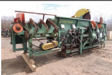
17099 MERCHANDISING SAW $27,500.00 Compact Maxi-Tour merchandising saw system, 72" dia blade, 75 hp electric drive, includes infeed/outfeed conveyors, 260-633-4047
