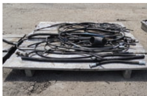
Hydraulic Hoses and Shaft 2 15/16" x 8' 6" shaft, assorted hydraulic hoses on skid
