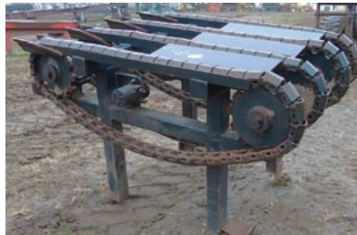
9202 TRANSFER DECK $1,500.00 4 strands, 3' wide x 4' 6" long, H-78 rooftop chain, no drive, excellent condition 260-633-4047
