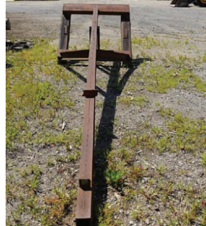
Jib Boom 20' boom, 47" between fork pockets, 7" pockets
