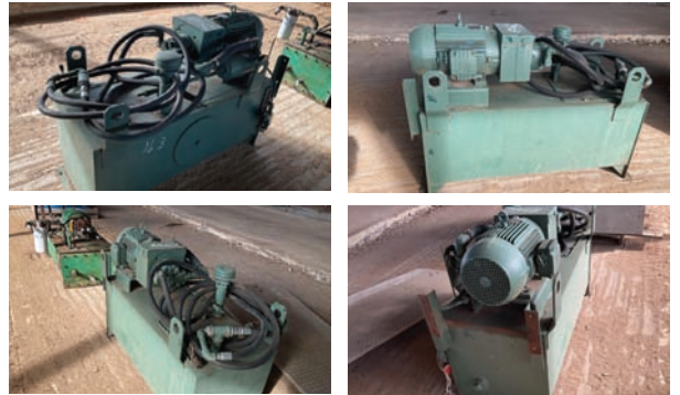
Hydraulic Pack 10 hp electric motor on pump, 48" x 18" x 20" tank.
