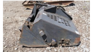
FFC Rockhound 76", hydraulic drive, skid steer quick attach
