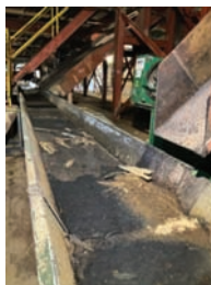
9256 VIBRATING CONVEYOR $28,750.00 Webster vibrating conveyor, 24" wide pan 9" tall sides, 80' long, electric drive, very good condition 260-633-4047
