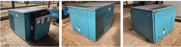
CompAir Screw Type Air Compressor Model 6000, 35 hp electric drive, meter reads 22455 hrs, has small oil leak, works.
