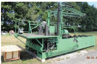
6031 $34,500.00 HMC DEBARKER rosser head style, all hyd. drive, 36" dia. log capacity x 12' long, very good condition 260-633-4047
