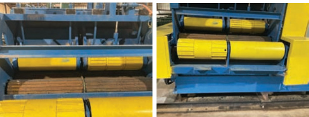
Tierney Gang Saw Edger Combo Serial #: 6-78-16. Model: na. # of Blades: not set up. # of Moveable Blades: 2. Arbor Size: 3 7/16". Blade Type: Circle. Cut Capacity: 24" gang side and 24" edger side. Drive Type: None. Edger Set Up: Stationary. Infeed Measurement: 54" x 12' live rolls and side shifting chains. Lasers: no. Outfeed Measurement: none. Features and Notes: Owner just put in and is not fully set up yet.
