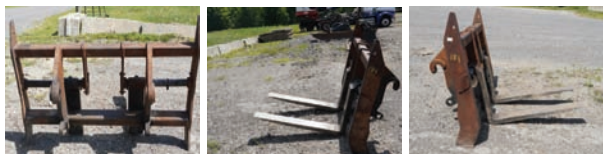
Loader Forks JRB quick attach 30 1/2" x 17", 6" x 44"
