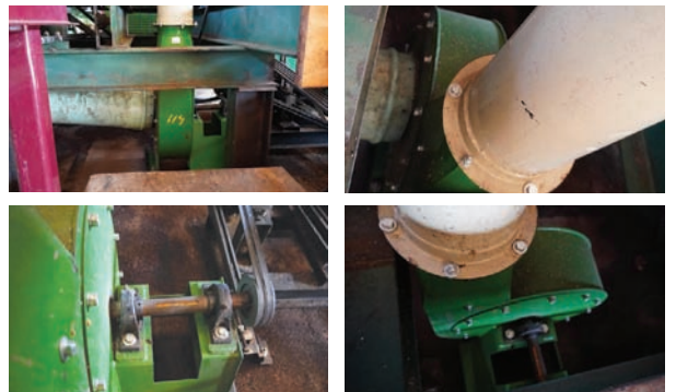
Dust Blower 24" blower, 10" inlet, 8" outlet, includes pipe adapter
