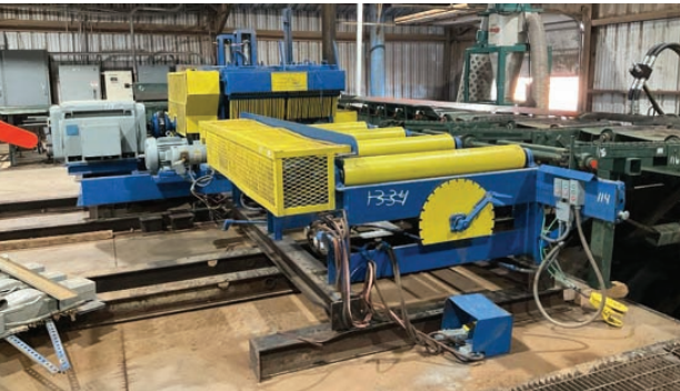
Tierney Gang Saw Edger Combo Serial #: 6-78-16. Model: na. # of Blades: not set up. # of Moveable Blades: 2. Arbor Size: 3 7/16". Blade Type: Circle. Cut Capacity: 24" gang side and 24" edger side. Drive Type: None. Edger Set Up: Stationary. Infeed Measurement: 54" x 12' live rolls and side shifting chains. Lasers: no. Outfeed Measurement: none. Features and Notes: Owner just put in and is not fully set up yet.
