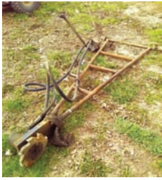
20280 MUD SAW $1,500.00 3/4" x 8" cutter, 6' arm, hyd drive, good working condition 260-633-4047
