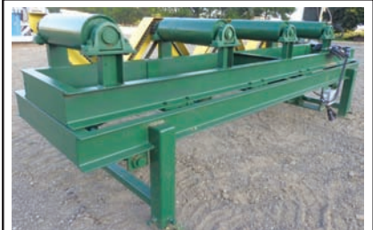
9217 ROLL CASE $4,500.00 pop-up rollers, perfect for putting in a transfer deck, 16" wide x 7' long, foot pedal control, hyd drive, BRAND NEW! 260-633-4047
