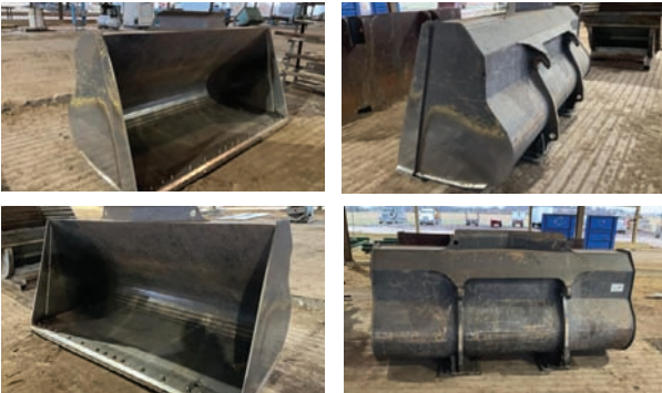
Volvo Bucket 3 yd capacity, 39.5" x 24" quick attach, bolted on cutting edge.
