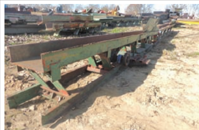
9078 $15,000.00 VIBRATING CONVEYOR Morbark 17" wide pan x 37' long, 6" tall sides, has fines section, chipper infeed spout, good condition 260-633-4047
