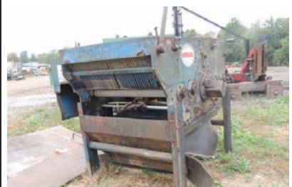
5116 BOARD EDGER $14,250.00 Cornell 4" thick x 27" wide capacity, 1 stationary-1 movable blade, includes infeed, this edger is in good working condition 260-633-4047
