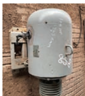
Lincoln Electric Motor Horsepower: 100. Frame Size: 405T. Phase: 3 Phase. RPM: 1765. Features and Notes: Good motor.
