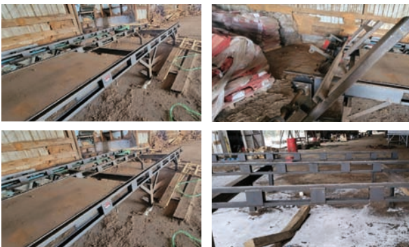
3 Strand Green Chain Model: Unknown. # of Strands: 3. Length: 80'. Width: 10'. Height: 30". Drive Type: Hydraulic. Rooftop Chain: No. Solid Decking: No. Features & Notes: Includes chain. Reassembled, ready to be loaded!
