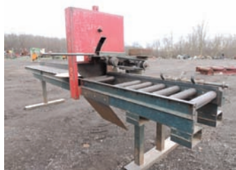
17095 CHOPSAW $7,500.00 Morgan chop saw, line shaft ready, 22" dia blade, includes 1 extra blade 10' infeed/5' outfeed, good condition and ready to work 260-633-4047
