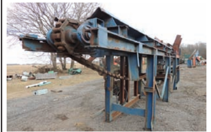
9232 $17,250.00 LOG TROUGH chain is 11" wide, trough is 38' long, electric gear box drive, 1 set of kickers, heavy duty and in good condition 260-633-4047
