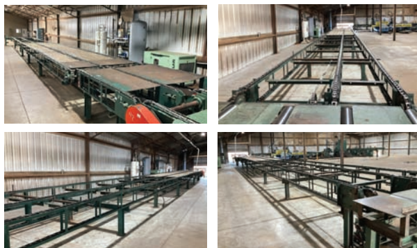
Green Chain Transfer Deck Model: na. Length: 70'. Width: 80". # of Strands: 3. Drive Type: Electric. Height: 39". Rooftop Chain: no. Solid Decking: yes. Features and Notes: Partial solid decking, deck is in 2 pc. Additional 2 strands to make 4' wider deck.
