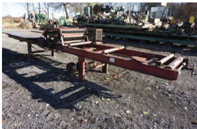
5130 EDGER $7,250.00 Meadows board edger, 4" thick x 66" wide capacity, infeed rollers, outfeed is a tilt table, line-shaft ready, 2 blades-1 is movable, good working condition 260-633-4047
