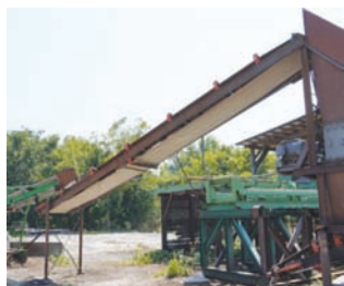
9219 CONCAVE BELT CONVEYOR $7,000.00 36" wide x 30' long, electric gear box drive, good working condition 260-633-4047
