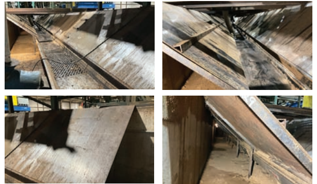
Slide Pan Slide pan along conveyor, 56" x 150'.
