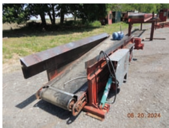
9180 DROP BELT $6,500.00 Slab drop belt, 24" wide x 12' long, electric drive, hyd cylinder for drop belt, includes hyd unit for cylinder, very good condition 260-633-4047
