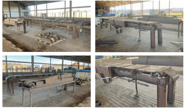
Rollcase with Popup Transfer Drive Type: None. Overall Dimensions: 28" x 22'. Roller Size: 5.5" x 18". Shaft Size: 1 7/16". Features and Notes: 4' 2 way popup transfer, 1 pc. 29" x 10' Rollcase no drive.
