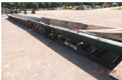
9183 VIBRATING CONVEYOR $16,000.00 Carrier vibrating conveyor, 24" wide pan x 50' long, 12" tall sides, electric drive, very good condition 260-633-4047
