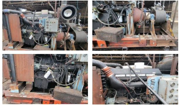
1995 Detroit 60 Series Power Unit SN: S4231. Meter reads: 4000 hours (not original hours). Horsepower: 450. Housing: Size 1. Clutch: Yes. Clutch Size: 14-3P. Fuel: Diesel. Voltage: None. Features & Notes: Twin disc. No blowby. This is a phenomenal power unit on a Rock Crusher base. This unit is in very good condition. It gave the seller no problems.
