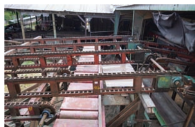
9225 TRANSFER DECK $4,500.00 4 strand transfer deck, 10' wide x 14' long, H-78 chain, gear box drive, good working condition 260-633-4047
