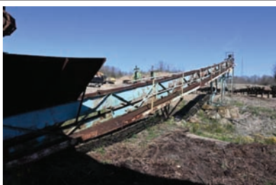
9025 $9,750.00 PADDLE CHAIN CONVEYOR 3" x 13" paddles, 16" pan, 15" sides, electric drive, 20" x 68' long, good condition 260-633-4047
