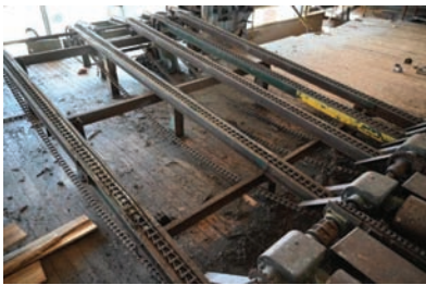
9018 $4,600.00 TRANSFER DECK 5 strand, 13' wide x 18' 6" long, H78 chain, electric drive, air cylinders on pop up board stop, good condition 260-633-4047
