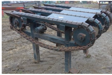
9202 $1,500.00 TRANSFER DECK 4 strands, 3' wide x 4' 6" long, H-78 rooftop chain, no drive, excellent condition 260-633-4047 WOLCOTTVILLE, IN
