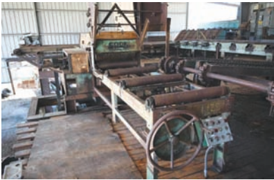
5114 $10,750.00 COOK EDGER Model:36EZTD, SN: 42, 5" x 21' tailing belt outfeed, 38" x 9' infeed rolls, 6" x 36" infeed cap, control panel, manual blade set, (2) 20" blades both are adjustable, electric drive, good heavy duty older unit 260-633-4047 WOLCOTTVILLE, IN
