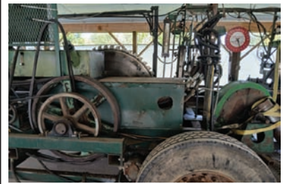
2101A $50,000.00 FRICK CIRCULAR MILL Portable, 3 head block, right hand, air dogs and flippers, hyd. networks and drive. This heavy duty mill is in excellent condition! The blade, blower, and the pipes are included. It was not used much after the track rails were replaced. 440-313-8683 MIDDLEFIELD, OH.
