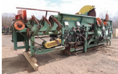
17099 $27,500.00 MERCHANDISING SAW Comact Maxi-Tour merchandising saw system, 72" dia blade, 75 hp electric drive, includes infeed/outfeed conveyors, 260-633-4047 WOLCOTTVILLE, IN
