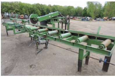
17104 CHOP SAW $12,500.00 for cants, 7" thick x 12' wide capacity, 18" wide x 14' long infeed, 18" wide x 10' long out feed, 2 air powered stops, cant pusher arms, shop built, line-shaft and air operated, good working condition 260-633-4047 WOLCOTTVILLE, IN
