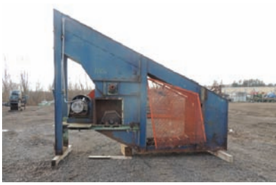
9250 $4,000.00 WASTE CONVEYOR ladderback chain, 18" wide pan x 33' long, 12" sides, electric gear box drive, was used on incline, good condition 260-633-4047 WOLCOTTVILLE, IN
