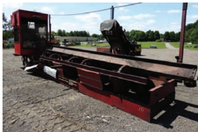
6046 DEBARKER $42,500.00 Mellott rosser-head debarker, your choice of power (electric or hyd), new babbit in bearings, new cleats on bull wheels, good condition and ready for production 260-633-4047 WOLCOTTVILLE, IN
