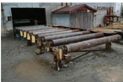
9229 ROLL CASE $15,000.00 90" wide x 28' long, electric drive, heavy duty and in good condition 260-633-4047 WOLCOTTVILLE, IN
