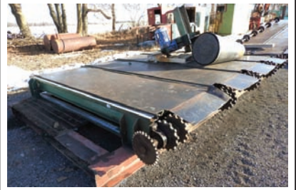
9252 $5,500.00 TRANSFER DECK heavy duty transfer deck, 5 strands, 14" wide x 12' long, electric drive, H-78 chains, very good condition 260-633-4047 WOLCOTTVILLE, IN
