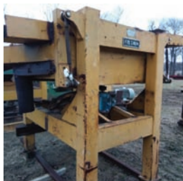
7085 FULGHUM SHAKER SCREEN $7,400.00 5' X 5' screen, electric drive, very good working condition 260-633-4047 WOLCOTTVILLE, IN
