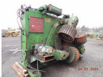
6045 RING DEBARKER $57,500.00 30" dia Cambio ring debarker, 6 arms, steel infeed press wheels, all electric, all electrical and controls included, recently in production and in good working condition, infeed/ outfeed also available, call for price 260-633-4047 WOLCOTTVILLE, IN
