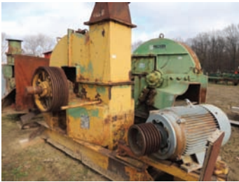
7138 CHIPPER $17,250.00 Fulghum 6 knife chipper, 60" dia, top discharge, working condition 260-633-4047 WOLCOTTVILLE, IN
