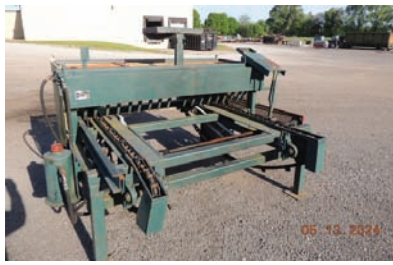
17105 DOUBLE END TRIM SAW $8,500.00 Morgan double end trim saw, 6" thick x 68" long capacity, line-shaft ready, feed is hyd driven, good operating condition 260-633-4047 WOLCOTTVILLE, IN
