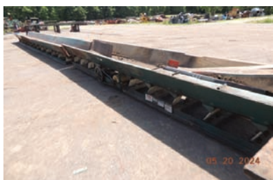
9183 VIBRATING CONVEYOR $16,000.00 Carrier vibrating conveyor, 24" wide pan x 50' long, 12" tall sides, electric drive, very good condition 260-633-4047 WOLCOTTVILLE, IN
