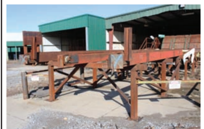
9266 $5,750.00 TRANSFER DECK 3 strand transfer deck, 10' wide x 18' long, 5 hp electric gear-box drive, 81X chain, good working condition 260-633-4047 WOLCOTTVILLE, IN
