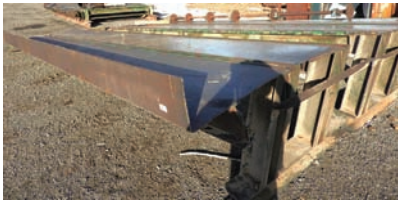
9253 $8,500.00 TRANSFER DECK 5 strand heavy duty deck, 12' 6" wide x 25' long, electric drive, H-78 chain, very good condition 260-633-4047 WOLCOTTVILLE, IN
