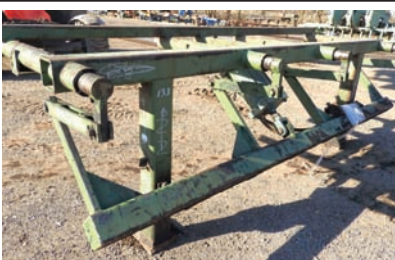
9244 CANT CATCHER $8,000.00 Reckart cant catcher for drop use with a drop belt, air powered, 4 arms, travel is 30", good working condition 260-633-4047 WOLCOTTVILLE, IN
