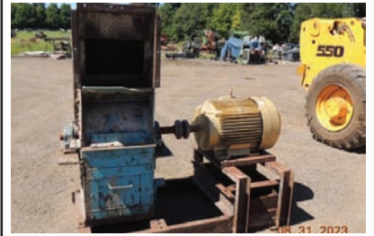
7134 WASTE GRINDER $6,300.00 Roberts hammer mill/ waste grinder, top feed, 60 hp electric drive, 3600 rpm's, good working condition 260-633-4047 WOLCOTTVILLE, IN
