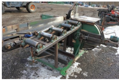
3096 $7,500.00 SINGLE HEAD RESAW Shop built Morgan style single head resaw, line-shaft ready, good working condition 260-633-4047 WOLCOTTVILLE, IN
