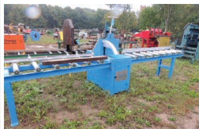
17094 $9,079.00 PROCUT CHOP SAW up-cut style, 7" x9" cutting capacity, 22" dia blade, includes 8' infeed/outfeed, 4 flip stops, BRAND NEW, buy this one or order one to your specs 260-633-4047 WOLCOTTVILLE, IN
