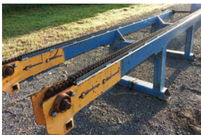
9216 TRANSFER DECK $2,500.00 2 strand transfer deck, 28" wide x 14' long, #80 roller chain, no drive, good condition 260-633-4047 WOLCOTTVILLE, IN
