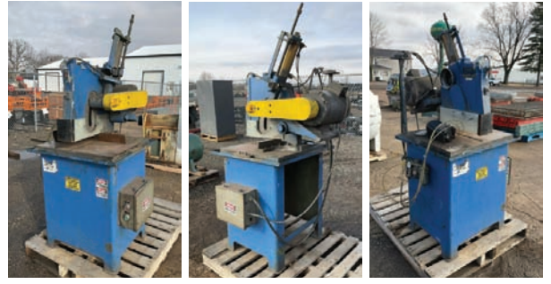
Steel SC16 Chopsaw SN: 5936. Blade Size: Approx 16" Diameter. Blade Drive: Electric. Blade Up/Down: Air. Cut Capacity: 12". Overall Machine Measures: 6' Tall x 35" Wide x 3' Deep. Features and Notes: Operating when uninstalled. Contact Zak with any questions, 260-221-2628
