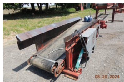
9180 DROP BELT $6,500.00 Slab drop belt, 24" wide x 12' long, electric drive, hyd cylinder for drop belt, includes hyd unit for cylinder, very good condition 260-633-4047 WOLCOTTVILLE, IN
