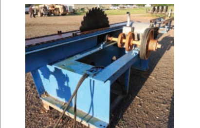
2094 $5,000.00 SPLITTER SAW designed to split cants, boards, etc., 50hp electric drive, 81x chain, 40" dia inserted tooth blade, hyd drive on feed, good working condition 260-633-4047 WOLCOTTVILLE, IN
