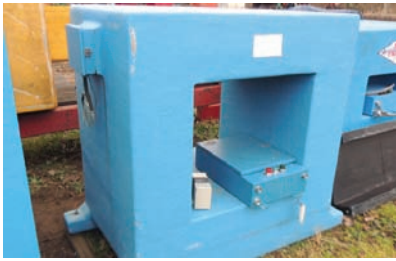
20270 $6,000.00 METAL DETECTOR MDI whole log metal detector, capacity is 30" wide x 28" tall, includes controls, very good condition 260-633-4047 WOLCOTTVILLE, IN
