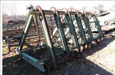
9230 TRANSFER DECK $3,000.00 7 strand, 12 1/2' wide x 7' long, 81X chain, electric drive, good condition 260-633-4047 WOLCOTTVILLE, IN
