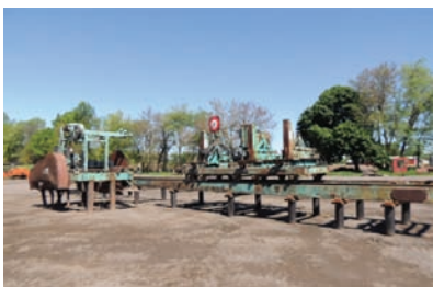
2091 $25,000.00 CIRCLE MILL Helle 3 head block, 36" carriage with 124" knees, husk with top saw, 60' long track, frame, 60 hp carriage drive, cab and all accessories, complete mill ready to work 260-633-4047 WOLCOTTVILLE, IN
