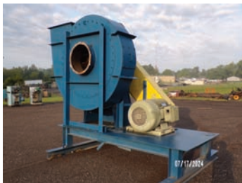
10366 $5,200.00 DUST BLOWER IAP dust blower, 24" dia inlet- 24" dia outlet, 150 hp electric drive, 18,000 cfm's very good condition 260-633-4047 WOLCOTTVILLE, IN
