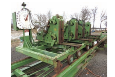
2096 $45,000.00 HMC CIRCLE MILL HMC 4 head-block circle mill, complete mill package, includes husk w/ top saw, carriage drive, operator cab, and all controls, price includes BRAND NEW set-works and mill gone through shop and ready for production 260-633-4047 WOLCOTTVILLE, IN
