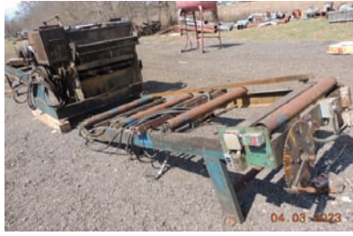
5111 $17,250.00 CORNELL EDGER 6" x 42" capacity, MN: HE42, SN: 703-10-81, single arbor, (4) 19" saws, 2 movable blades, 8' infeed, 8' powered outfeed, electric drive, comes w/ spare spacers, saws and laser lights 260-633-4047 WOLCOTTVILLE, IN
