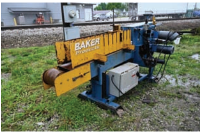
14080 DEDUSTER $10,000.00 Baker board deduster, up to 8" wide capacity, electric drive, price includes all new brushes, feed belt and gone through completely, very good condition 260-633-4047 WOLCOTTVILLE, IN
