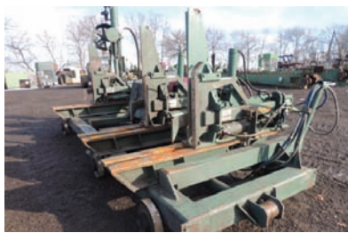
2088 $47,500.00 CLEEREMAN CARRIAGE Cleereman 3 head-block carriage, Silva-Tech computerized set-works, 48' long track/frame, incudes cab, drive, husk and all controls, good working condition 260-633-4047 WOLCOTTVILLE, IN
