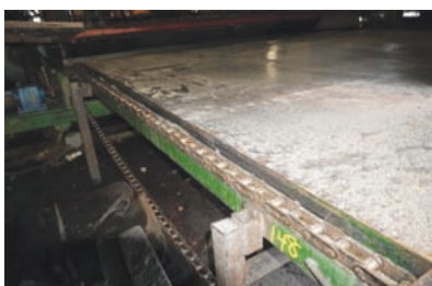
9223 SLAB DRAG DECK $8,500.00 slab drag conveyor, 15' x 14', electric gearbox drive, 81X chain with steel cleats bolted on, good condition 260-633-4047 WOLCOTTVILLE, IN
