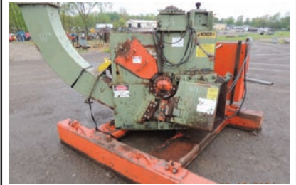
7148 CHIPPER $32,500.00 48" 6 knife chip-pac, includes 5' x5' shaker screen, electric drive, includes soft start, numerous spare knives and parts, good working condition 260-633-4047 WOLCOTTVILLE, IN
