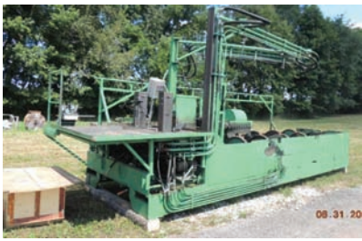
6031 HMC DEBARKER $34,500.00 rosser head style, all hyd. drive, 36" dia. log capacity x 12' long, very good condition 260-633-4047 WOLCOTTVILLE, IN
