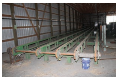
9265 $13,500.00 GREEN CHAIN 5 strand green chain, 11' wide x 65' long, electric gear-box drive, C-55 rooftop chain, excellent condition 260-633-4047 WOLCOTTVILLE, IN
