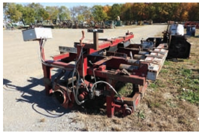
14081 NOTCHER $22,500.00 Keystone double head notcher, electric drive on heads, hyd's for pusher arm, good working condition 260-633-4047 WOLCOTTVILLE, IN
