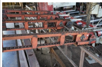
9222 TRANSFER DECK $3,750.00 4 strand transfer deck, 10' x 10', H-78 rooftop chain, hyd drive, air powered board stops, good condition 260-633-4047 WOLCOTTVILLE, IN
