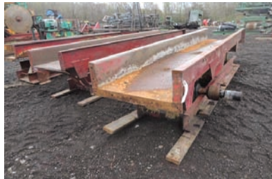
9236 VIBRATING CONVEYOR $10,500.00 30' L, hyd drive, 24" pan, 8" sides, 19" from floor to bottom of pan, good condition 260-633-4047 WOLCOTTVILLE, IN
