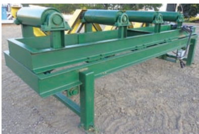
9217 ROLL CASE $4,500.00 pop-up rollers, perfect for putting in a transfer deck, 16" wide x 7' long, foot pedal control, hyd drive, BRAND NEW! 260-633-4047 WOLCOTTVILLE, IN
