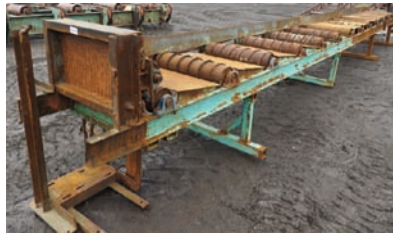
9259 $4,250.00 ROLL CASE 24" wide x 25' long, 6" dia rolls, good working condition 260-633-4047 WOLCOTTVILLE, IN
