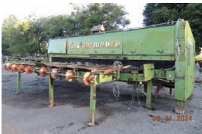
17112 TRIMMER $17,500.00 drop trimmer, 9 blades, up to 18' long capacity, air cylinders on heads, electric powered, price does not include going through shop 260-633-4047 WOLCOTTVILLE, IN
