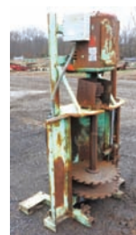
5131 VERTICAL EDGER $12,500.00 Helle 2 blade vertical edger, 22" dia blade, 40 hp electric drive, price includes going through shop, good working condition 260-633-4047 WOLCOTTVILLE, IN
