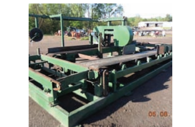
3087 $40,000.00 GRADE RESAW "Hochstetler" band resaw, 12" x 12' long capacity, 2" x 30" band wheels, line-shaft ready, foot print 11'6" wide x 28'6" long, complete run-around system ready to work, very good condition 260-633-4047 WOLCOTTVILLE, IN
