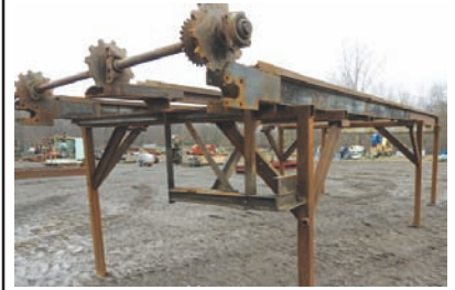
9260 $1,850.00 TRANSFER DECK transfer/ log deck, 3 strands, 8' wide x 20' long, H-78 chains, working condition 260-633-4047 WOLCOTTVILLE, IN
