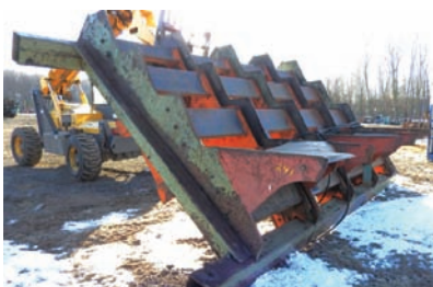
9264 $22,500.00 STEP FEEDER Linden step-feeder for logs, 16' long capacity, 15 hp electric powered hy unit, good working condition 260-633-4047 WOLCOTTVILLE, IN
