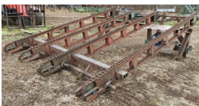
9225 TRANSFER DECK $4,500.00 4 strand transfer deck, 10' wide x 14' long, H-78 chain, gear box drive, good working condition 260-633-4047 WOLCOTTVILLE, IN
