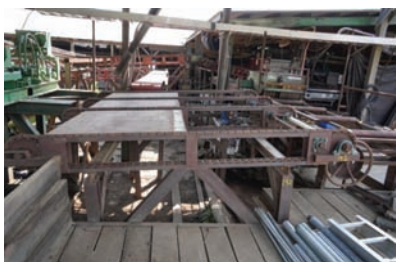
9227 TRANSFER DECK $3,750.00 4 strand transfer deck, 10' 6" x 10' long, H-78 rooftop chain, electric gearbox drive, has board stops, good condition 260-633-4047 WOLCOTTVILLE, IN
