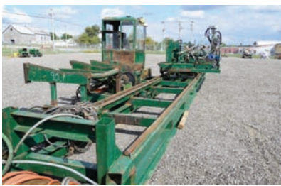
2087 $20,000.00 HMC 4 HEAD BLOCK CARRIAGE HMC HC-40, serial #330-1982, 4 head-block carriage, 110 volt electric over air set-works, 50 hp carriage drive, air powered dogs, 40' long track, was used with band head, includes cab, controls and log turner, complete unit ready to operate and in good condition 260-633-4047 WOLCOTTVILLE, IN
