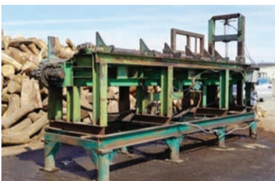
9238 LOG TROUGH $14,300.00 50"x 22' overall, air cylinder log clamp down, electric drive, WR124 chain w/cleats, air cylinder on loader 260-633-4047 WOLCOTTVILLE, IN
