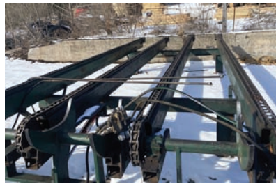
9607 MELLOTT LOG DECK WITH STOP & LOAD $12,000.00 Heavy duty, all hyd., 4 strand, 10' x 26' long, hyd. controls included. 7 years old and in very good condition. 717-250-7778 MCallISTERVILLE, PA.
