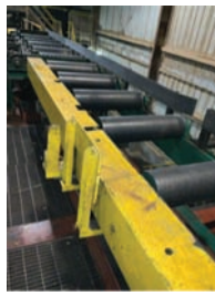
9251 $8,500.00 ROLL CASE 30" wide x 35' long, 8" dia rolls, electric drive, includes 4 strand pop-up transfer that is electric drive, this unit is heavy duty and in very good condition 260-633-4047 WOLCOTTVILLE, IN
