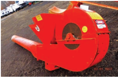
10211 MORBARK CHIP BLOWER $3,450.00 30 in. dia. 15 HP. electric motor, includes mounting plate and pipe, VERY GOOD CONDITION 260-633-4047 WOLCOTTVILLE, IN
