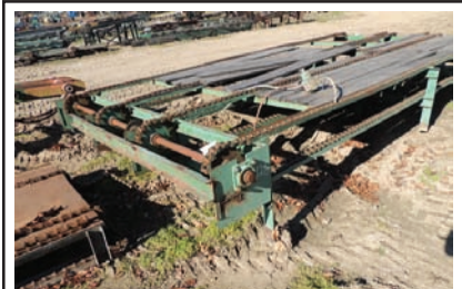
9249 TRANSFER DECK $5,000.00 4 strand, 10' wide x 22' long, H-78 chain, good condition 260-633-4047 WOLCOTTVILLE, IN
