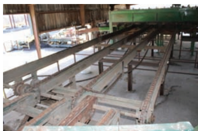
9268 $8,500.00 TRANSFER DECK 4 strand transfer deck, 10' 5" wide x 35' long, electric gear-box drive, 81X chain, good working condition 260-633-4047 WOLCOTTVILLE, IN
