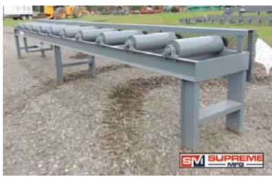
9129 $10,750.00 SUPREME MFG ROLLCASE 20" wide x 20' long, 6" dia rolls, 1 7/16" dia shafts, electric drive, BRAND NEW!! 260-633-4047 WOLCOTTVILLE, IN
