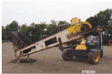
9206 $3,500.00 BELT CONVEYOR cleated belt conveyor, 24" wide x 18' long, set up for incline, electric drive, excellent condition 260-633-4047 WOLCOTTVILLE, IN
