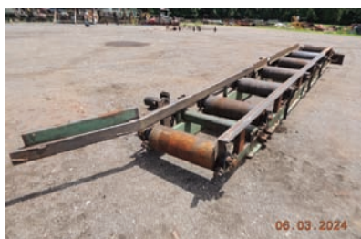
9192 ROLL CASE $3,500.00 24" wide x 19' long, 8 1/2" dia rollers, hyd drive, heavy duty and in good working condition 260-633-4047 WOLCOTTVILLE, IN
