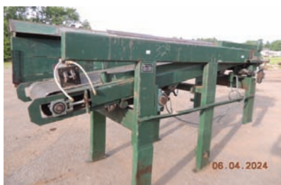
9191 DROP BELT $9,500.00 Pendul slab drop belt, 24" wide x 10' 6" long, hyd drive, twin air cylinders for up-down on belt, heavy duty and in excellent condition 260-633-4047 WOLCOTTVILLE, IN
