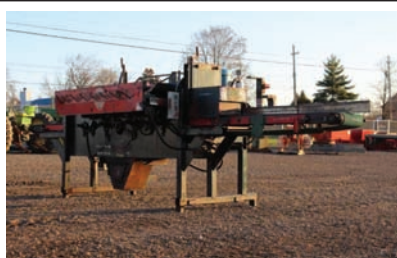
4035 $17,250.00 GANG SAW Morgan single arbor gang saw, capacity 12" wide x 5 1/2" thick, 100 hp electric drive on arbor, feed rolls are hyd drive, includes spare spacers, could be used for scragg slab edger, good condition and ready to work 260-633-4047 WOLCOTTVILLE, IN
