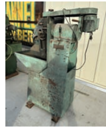
15604 CIRCLE SAW GRINDER $800.00 3 phase, 110V, will grind 24" - 30", will do alternate bevel, good condition 530-218-4471 RICHMOND, CA
