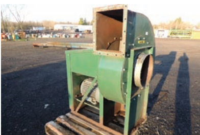
10359 $2,500.00 BLOWER 36" dia dust blower, 20 hp electric powered, 14" inlet- 12"x15" outlet, excellent condition 260-633-4047 WOLCOTTVILLE, IN
