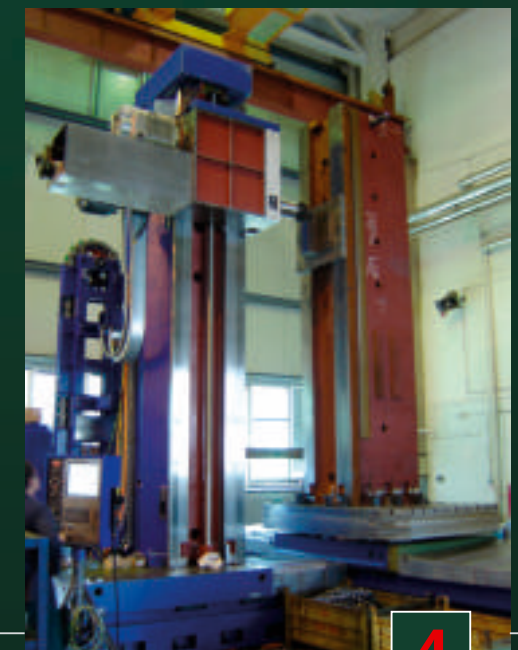
Machining check of machine with maximum feed and load
