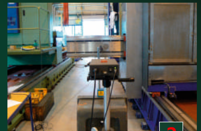
Test of accuracy in positioning (measuring by the laser)
