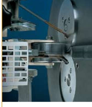
Tolerance compensating mechanism for different veneer thickness.
