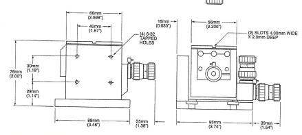
The MDT Series Flexure Stages are designed using precision components which provide the ultimate translator design for high precision applications. The primary drawback of the flexure design is a limited range of motion; our MDT Series provides 2mm of travel in a package that ensures long term stability. These stages find many applications in fiber optic positioning and the life sciences as micropositioners capable of nanometer level displacements.
