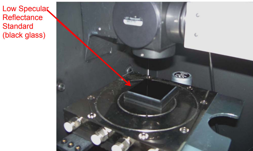
Figure 72: Low Specular Reflectance Standard During Calibration
