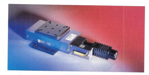
The UZM Series linear stages offer high-precision vertical translation for applications requiring submicron resolution. Their low-profile design makes them particularly suited for space-limited XYZ positioning applications. Unlike vertically-mounted linear stages, UZM Series stages center payload mass directly over the bearings, avoiding positioning errors caused by cantilever loads.
