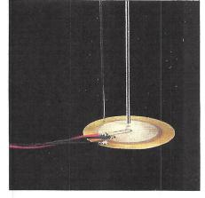
Two fiber-optic probes are used to measure surface displacement of a ceramic resonator. Fotonic probes are immune to electromagnetic interference (EMI) and operate effectively on a wide range of surfaces including nonmetallic materials, ceramic, glass, plastics, and composites.
