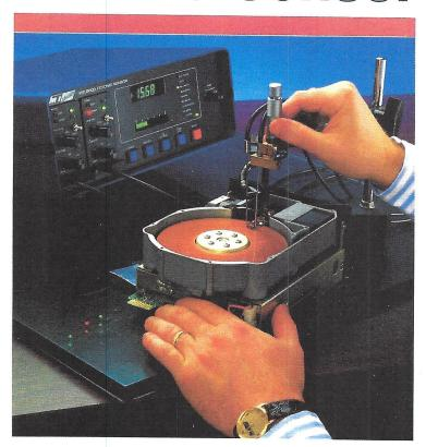
High-resolution, noncontact measurement of vibration and displacement
