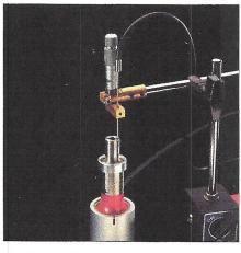
The Fotonic Sensor accurately measures the vibration amplitude of an ultrasonic welder tip at high frequencies and accelerations.
