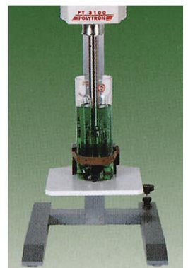
Lift the dispersing vessel into work position with the work table of the stand PT-ST 3001
