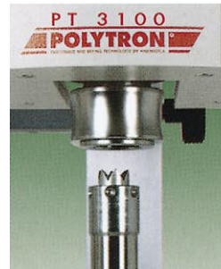
Lock the dispersing aggregate to the drive unit with the safety quick-coupling
