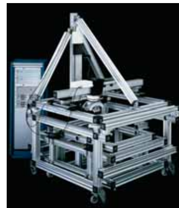
An ultra-sound non-destructive testing system built with X95 rails and Newport positioning equipment
