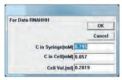
The concentration (*C in Syringe (mM)*) and *C in Cell (mM)*) values displayed are those entered by the operator before the experiment starts. Cell volume (*Cell Vol. (mI)*) is constant, which is stored in the data collection software. This value is read by Origin whenever an ITC data file is opened.
