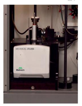
MicroCal Auto-iTC $_{200}$  is composed of the calorimeter, a fluidic system, autosampler, and temperature-controlled tray for storing samples. A computer controller is provided with the instrument and contains proprietary software and calibration constants specific to the automation and MicroCal iTC $_{200}$ . A set of reagent (water, detergent, and methanol) bottles, a waste bottle, and a nitrogen tank are plumbed to the rear of the Autosampler.
