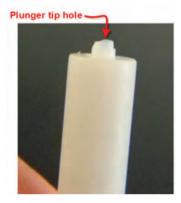
14 Insert the tip pusher and new tip into the pipette and press the tip into place.
