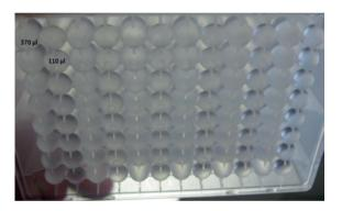
Cover the microtiter plate with a ZoneFree cover (Part No. 28429092) or a Biacore 96-well Microplate Foil (Part No. 28975816). Be careful to center the holes in the cover over the plate wells.
