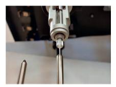
7 Grab the syringe bore firmly and pull straight down to remove the syringe from the pipette. The soft-grip tweezers can be used to help grip the syringe without damaging it. Set the syringe aside.
