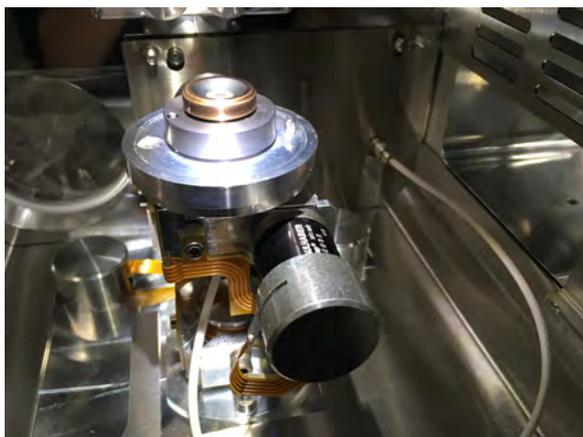
Connect the plug of quartz measuring cable to the feed through in the rear right of the coating chamber.
