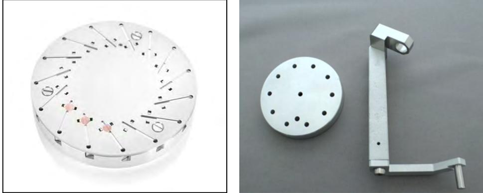
Standard stage and quartz holder mounted on the EM ACE600
