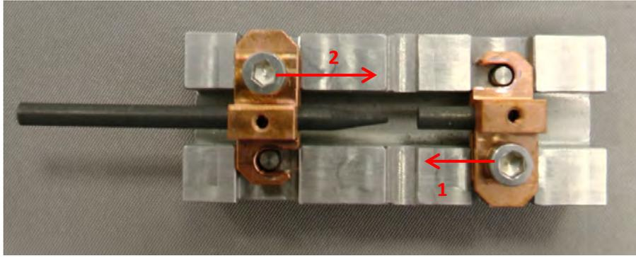
Firmly tighten the screws, but do not overtighten.
