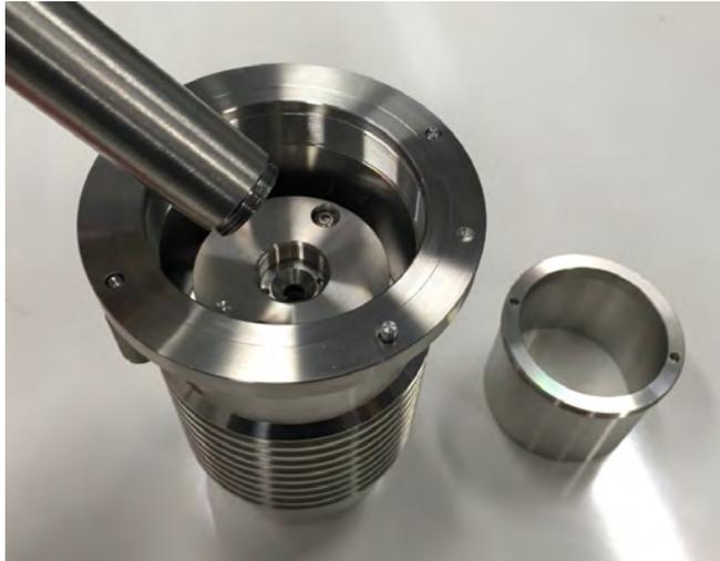
Pull upwards to get the e-beam source out of the housing.
