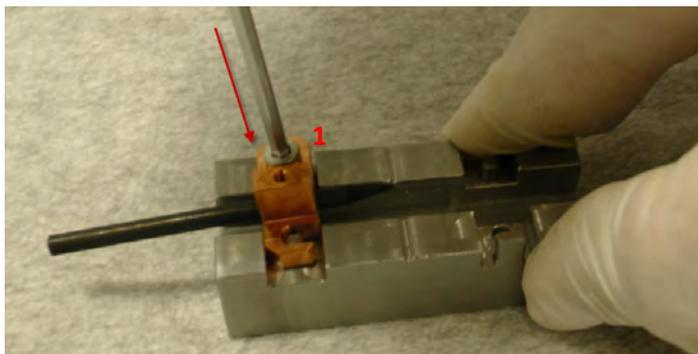
Use the special tool to keep the carbon rod evaporation source (spring loaded) open.
