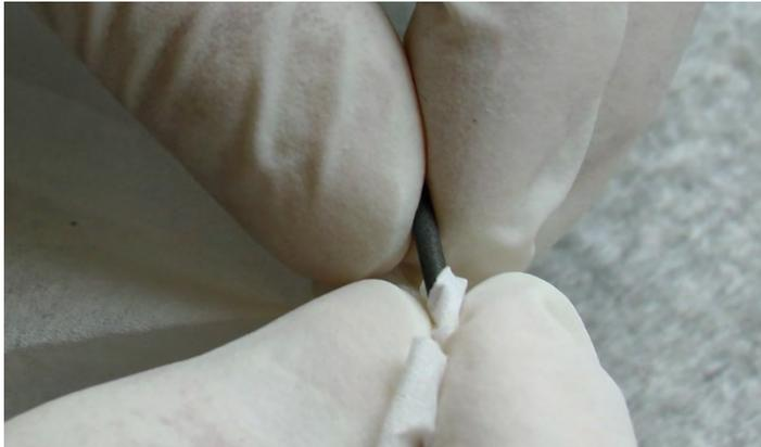
The platinum carbon rod is prepared for melting in (degassing, image shows a melted in rod).
