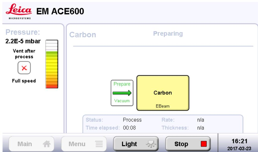
Tapping on the process box (Carbon in this case) shows the most important parameters of that process.
