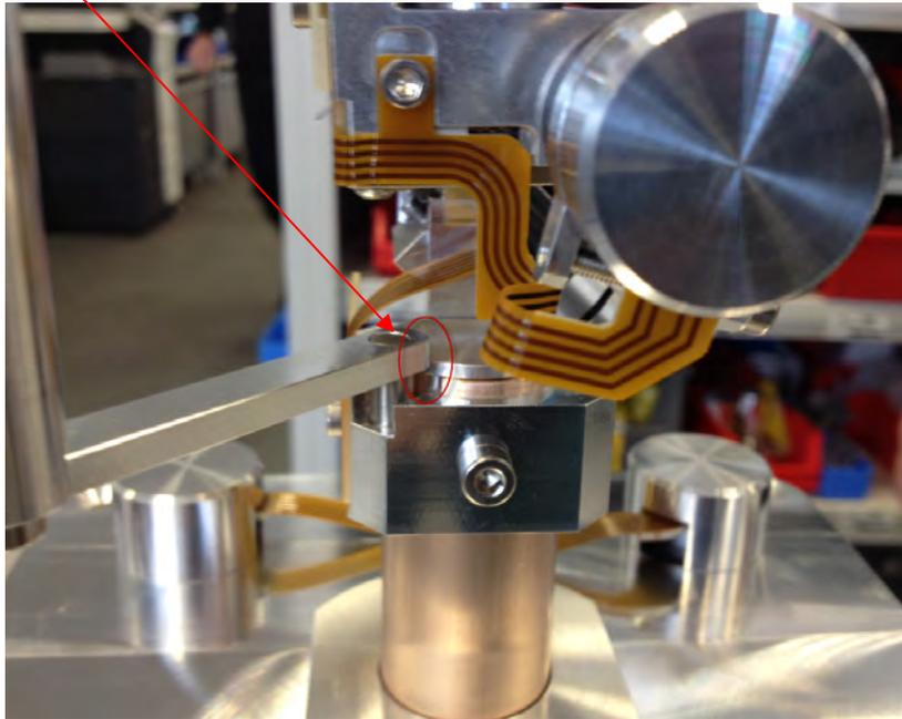
Loosen the screw with an Allen key and lift up the cover slightly, the stage will slide in.
