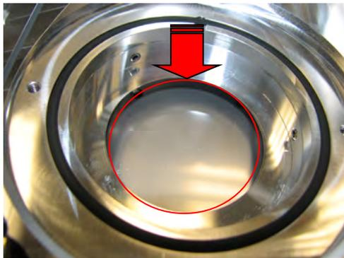
Occasionally, it can happen that an elongated flake builds up by the sputtered material. This can cause a short circuit that will be indicated by a warning when starting a sputtering process. Clean the anode ring by wiping with ethanol.
