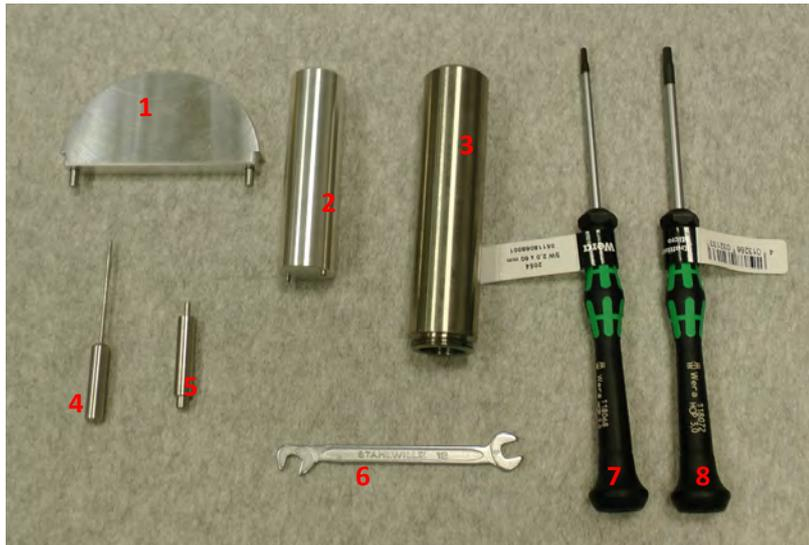
1. Special tool to unscrew the holding ring
