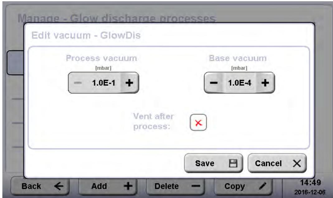
60 seconds @ 15 mA at 4E-1 mbar (1E-3 mbar Pre-Process- Vacuum) guideline for glow discharging grids to make them hydrophilic.
