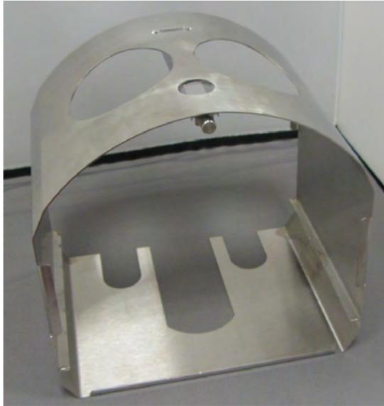
Take out the main shielding and unscrew the screw on the top middle of the chamber shielding which holds the part to separate and close the gap between the two shutters.
