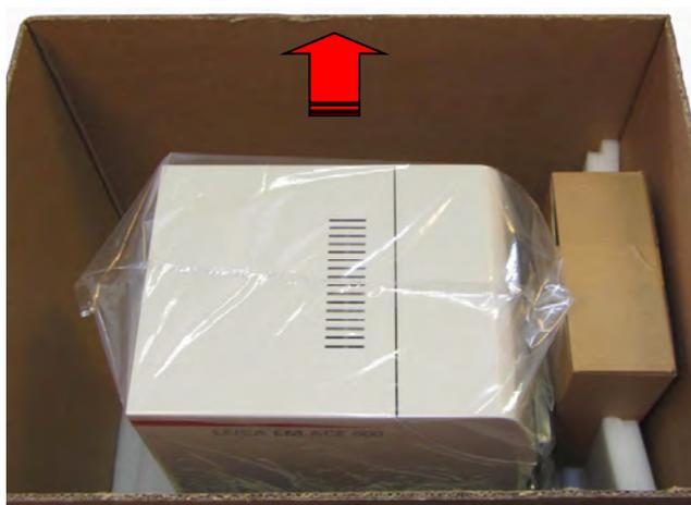
Lift out the unit by grasping underneath the back and the front as indicated in the picture (packaging provides recess for hands) and place it on a table. Two strong people are required to lift the coater!
