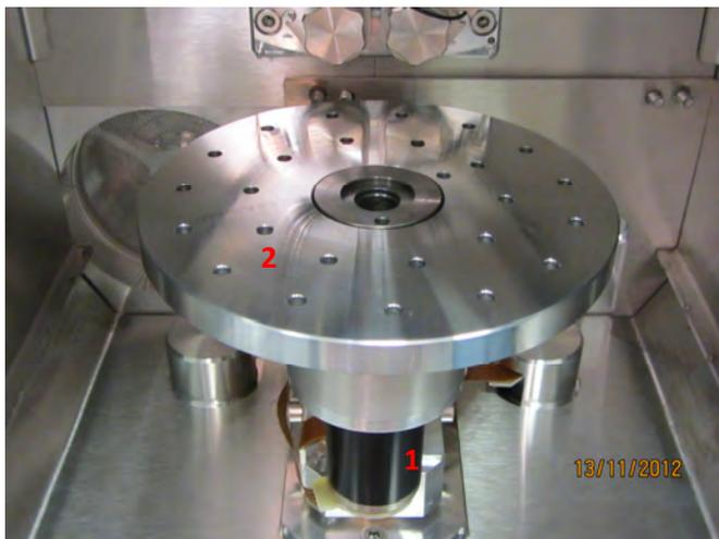
The optional table is used for two 76 mm x 26 mm (3" x 1") standard glass slides.
