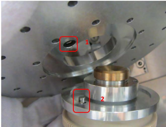
Motorized stage (1) with table (2) to load up to 24 standard 12.7 mm (1/2") SEM stubs with a pin diameter of 3.2 mm.
