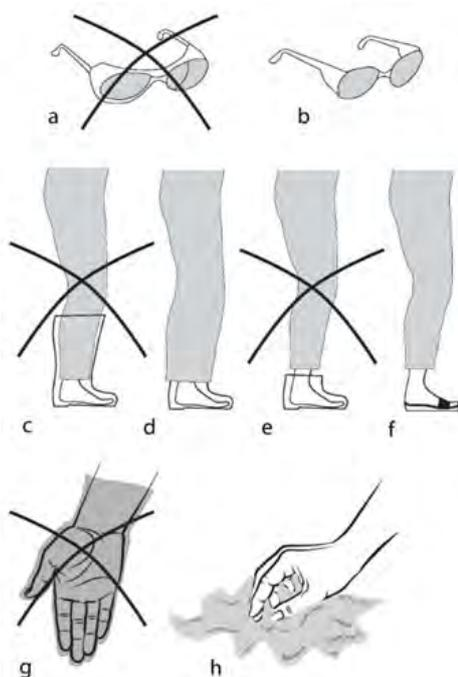
**Fig.1.1:** When working with  $\text{LN}_2$  for refilling the Dewar avoid protective glasses (a), boots (c), walking shoes (e) and protective gloves (g) out of which the  $\text{LN}_2$  cannot easily escape if entered.  $\text{LN}_2$  splashing into the closed protective glasses (a), open boots (c), shoes (e) or protective gloves (g) evaporates suddenly and can cause serious burns.
