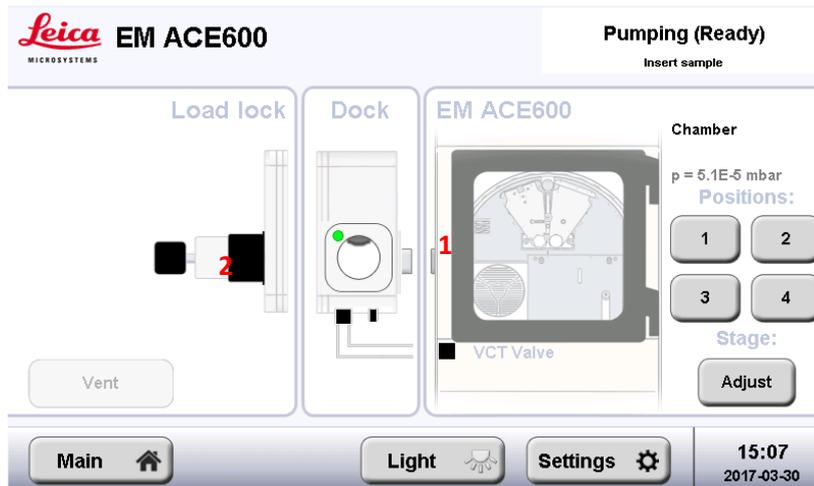
After placing all the samples (up to four), the load lock manipulator has to be pulled out. It is recommended to close the gate valve after finishing load lock manipulation. With the button Vent, the gate valve is closed.
