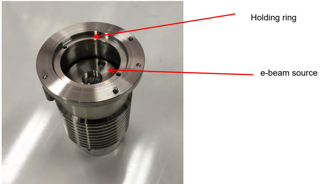
Use the special tool to unscrew the holding ring.
