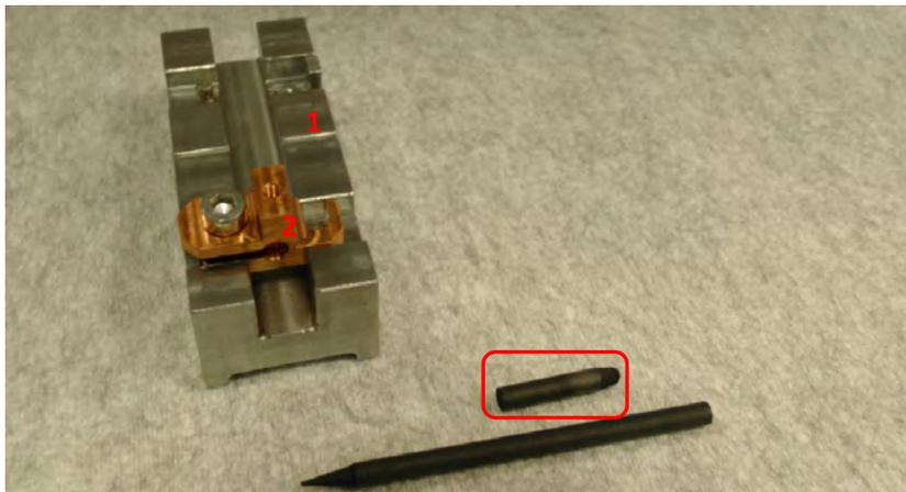
On the shorter side (1) mount the flat rod, aligned with the edge of the recess. On the longer side (2) mount the pointy rod, the tip aligned with the edge.
