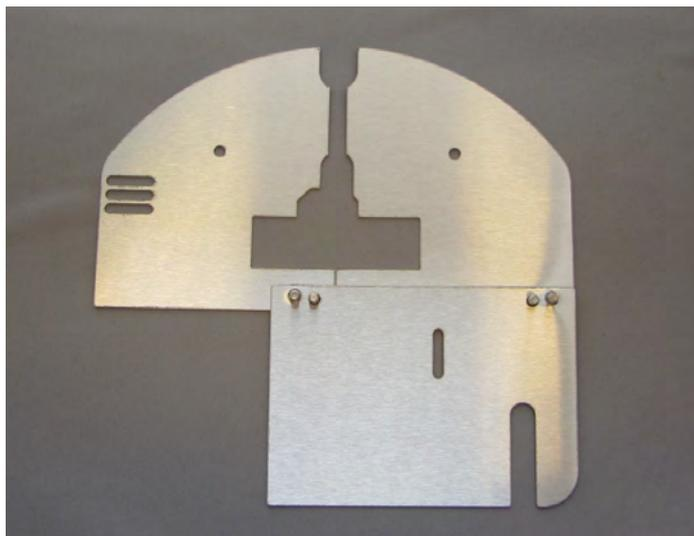
The first shield goes into the right top corner of the rear of the coating chamber. Align hole to the pin on the chamber wall and push on.
