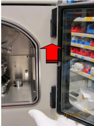
Place the door flat on a soft surface to clean. Do not use abrasive cleaning material. Scratches could cause a vacuum leak.
