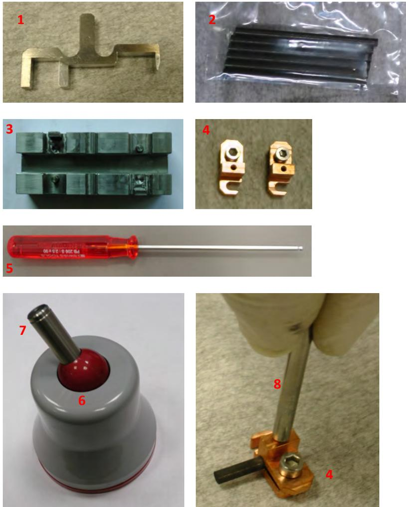
1. Special tool to keep the carbon rod evaporation source open for mounting
