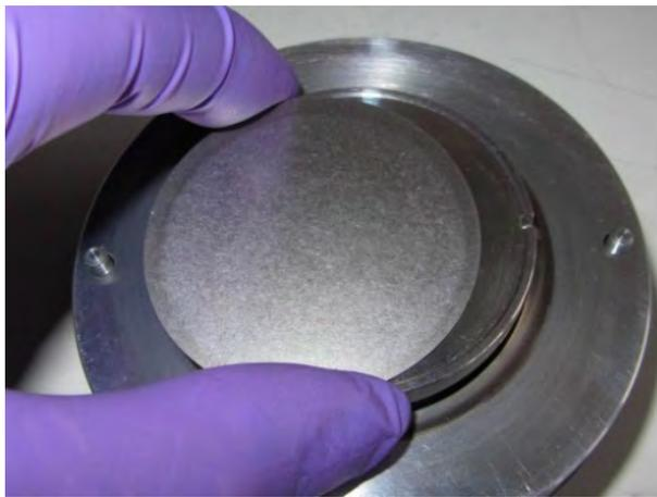
Fix target by gently tightening the bayonet ring.
