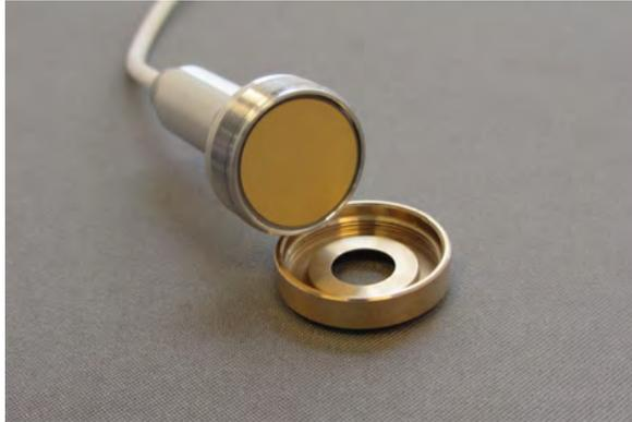
Slide quartz (1) from the top through the hole (2) in the middle of the stage.
