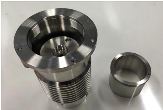
Use the special tool to take out the e-beam source, by screwing it into the thread in the middle.
