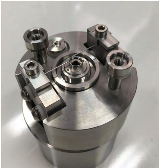
Put the Wehnelt cylinder on top and fix it with the two screws.
