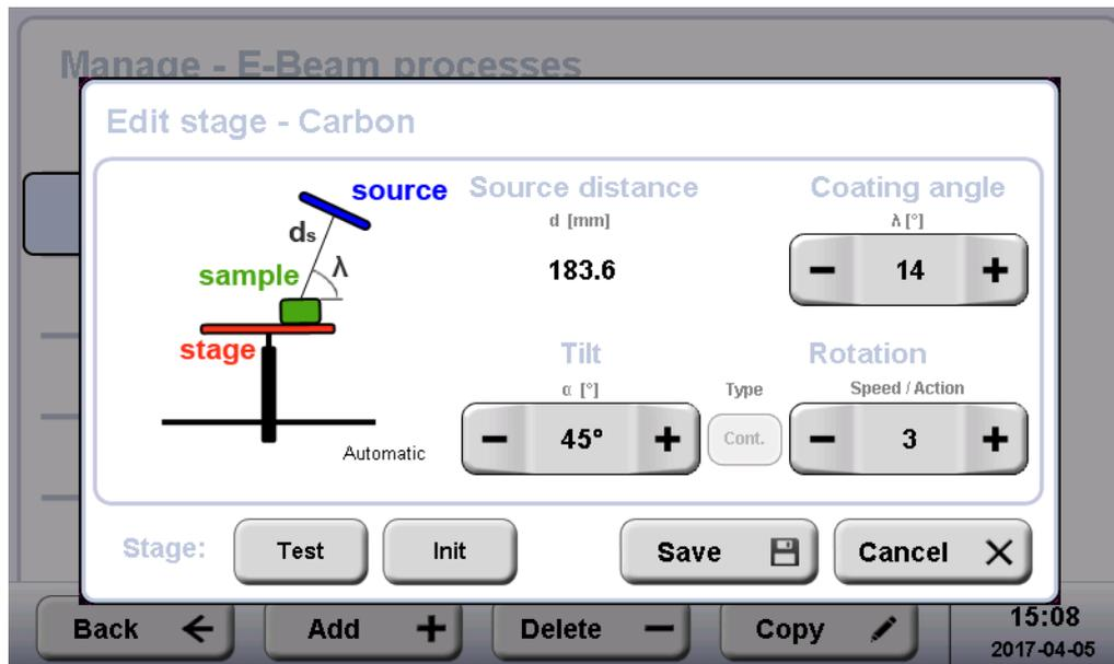
Note: Source distance is the real distance from sample to the evaporated material. Working distance is the vertical line from the horizontal table to the Wehnelt cylinder.
