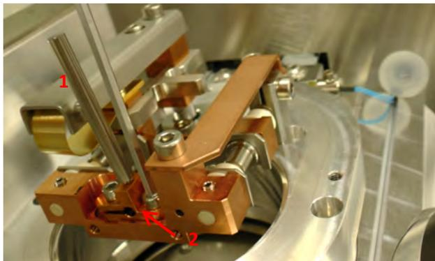
When the second rod is mounted in the same way the tool, which keeps the evaporation source, open is removed (1). The two rods should push against each other (2).
