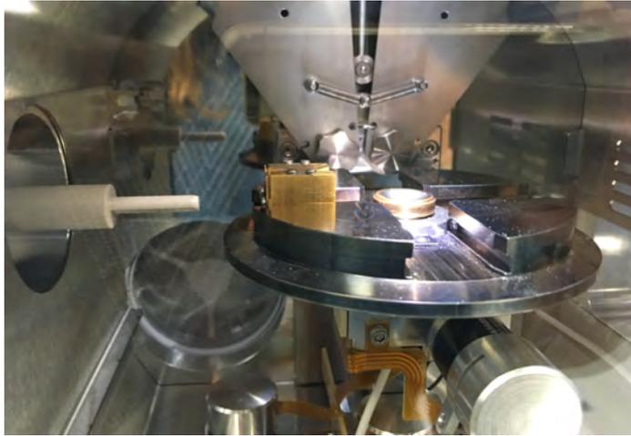
Select transfer on the first screen to enter the load lock operating panel. This screen is only accessible when the pressure is lower than 1,0E-4 mbar.
