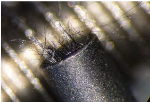
Rubbing with a lint-free paper over the surface will remove all the fibers. The platinum pellet is now fixed into the rod and ready for melting in.
