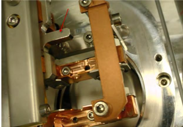
With the help of the holding pin (1) which is screwed into the clamps, the carbon rod can be easily loaded in the evaporation source. Make sure the clamp (2) sits straight in the recess and firmly tighten the screw. It is recommended to start with the flat rod on the front side in respect to the instrument.
