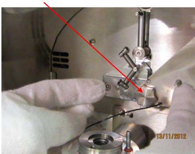
If a glow discharge is present, lace guide the cable through the recesses on the shutter (1) and plug in the connection (2).
