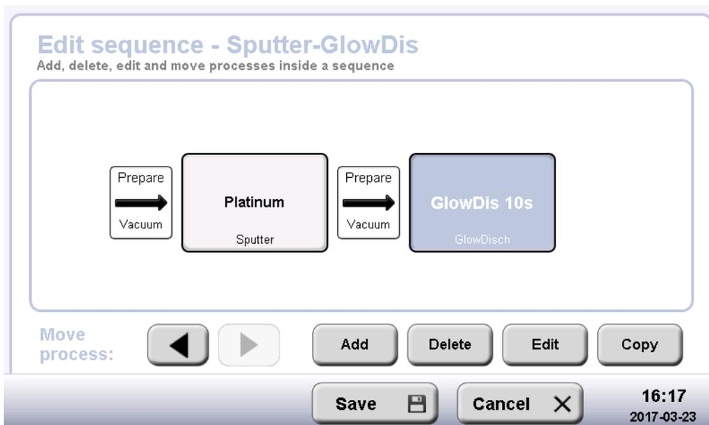
Tapping on an already implemented process allows changing the process itself or moving the position.
