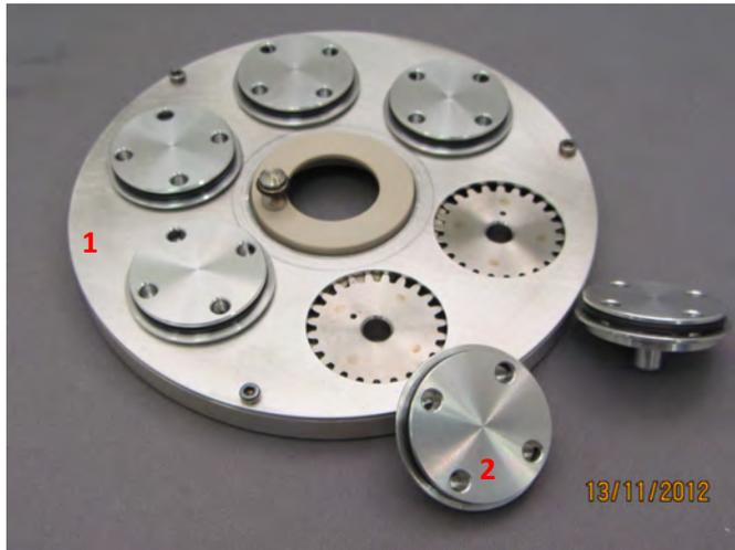
The planetary table is placed on the stage connecting first the screw (1) with the threaded hole, then turning the table until the pin on the table connects with the hole on the stage. Then, gently tighten the small thumbscrew (1).
