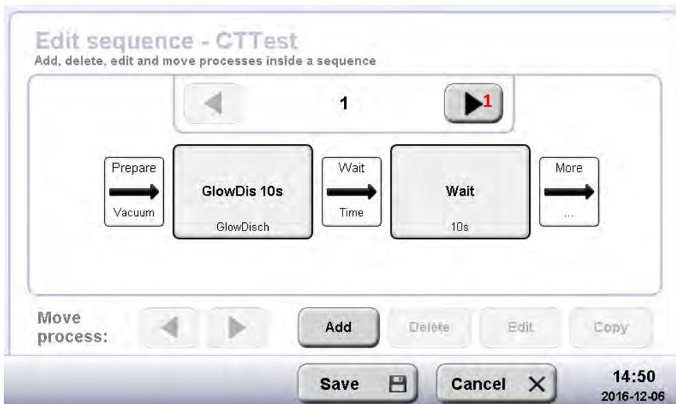
Tapping on add, a new process can be implemented into the sequence. First the method is selected, then the specific protocol and then the position in the sequence.
