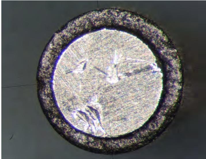
Method 3: Glue the pellet with some carbon cement into the carbon rod. A tooth pick or similar and forceps are needed.
