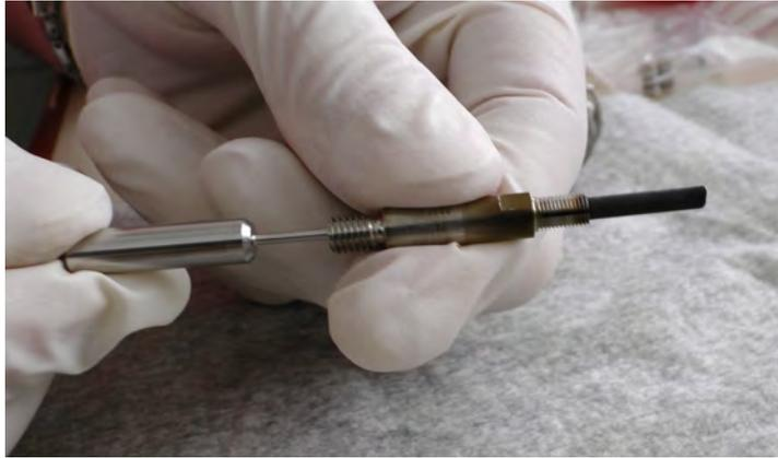
To prepare a carbon rod take a new rod and cut it in half. Use a razor blade to score the middle. After scoring the surface...
