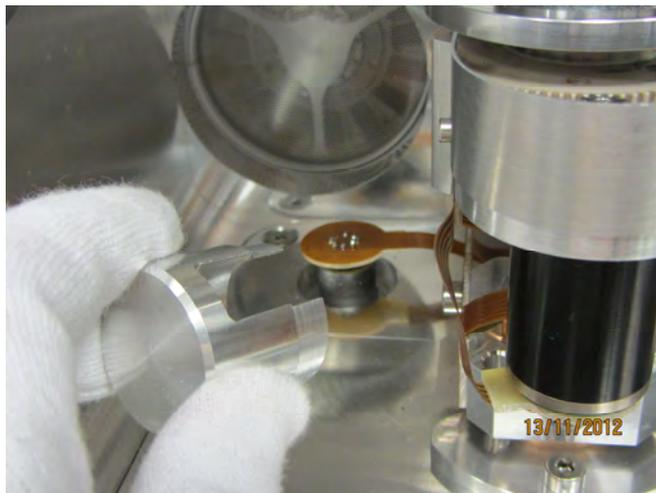
The motor spindle is covered and secured with a screw.
