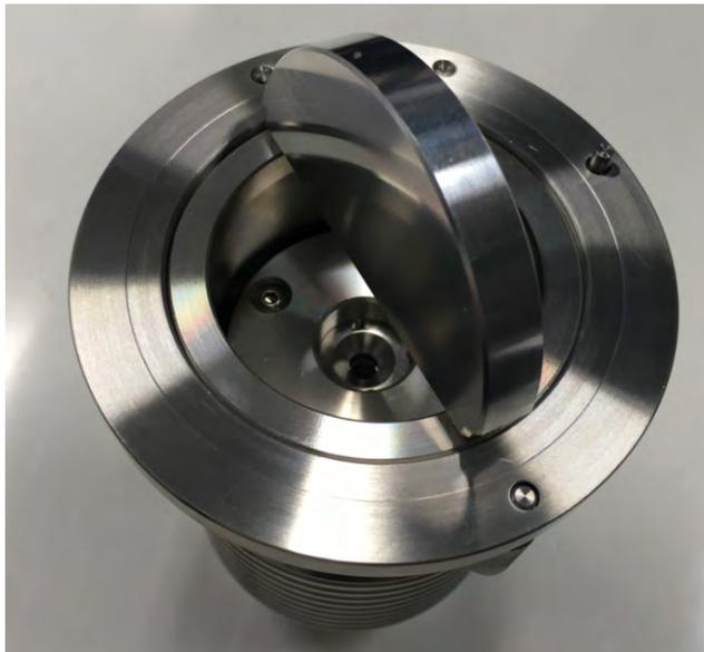
Remove the holding ring and place the holding ring next to the e-beam source.
