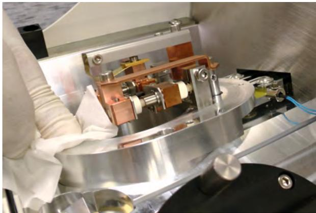
Reattach the source cover, tighten the evaporation head screws and close the cover.
