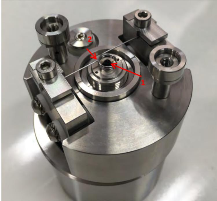
To change the carbon rod, screw out the collet holder.
