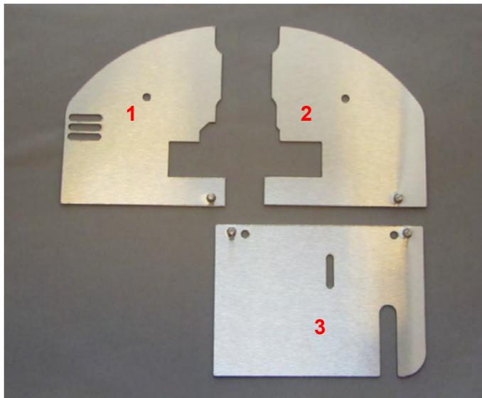
The three plates fit together in the rear of the coater like as shown here:
