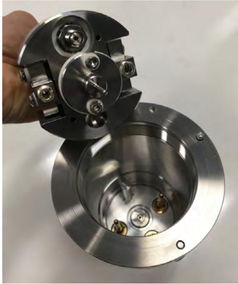
Push in so all the contacts are closed and screw in the holding ring.
