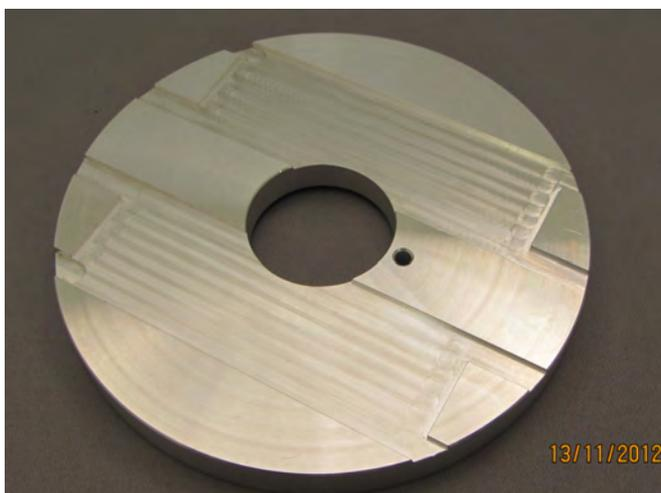
The optional **planetary table** (1) can hold up to 24 standard 1/2" SEM stubs (six planets (2) receiving 4 SEM stubs each).
