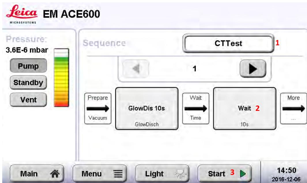
Select a protocol for a sequence by tapping on it. Once it is marked by tapping on the name or included processes, the details can be changed. Alternatively, a sequence can be copied and then modified or a new one added.
