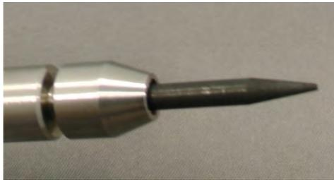
Take the alignment tool (1) and put in the first copper clamp (2). As shown on the image, a rod, which cannot be used for the sharp tip anymore, can still be used on the flat side.
