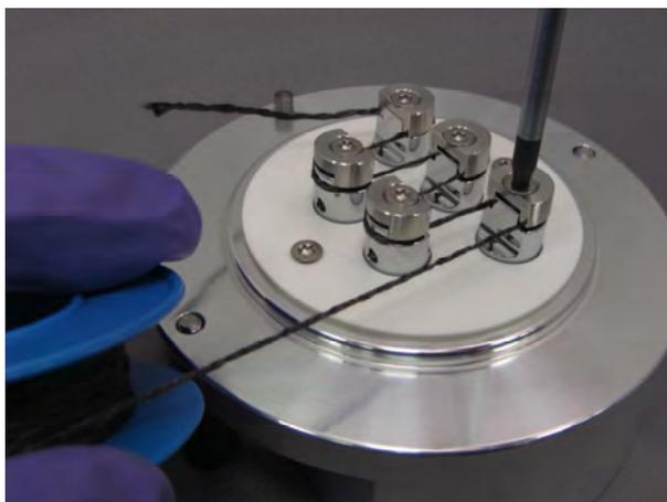
Tighten the remaining 3 screws and trim thread on both ends.
