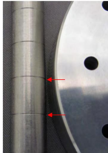
Stage on the lowest position equals to a source distance of 100 mm.
