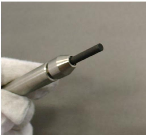
Turn the carbon rod holder in circles until the top is sharp. Flatten the tip to about 1 mm diameter. This will allow an exact positioning against the flat rod for evaporation.
