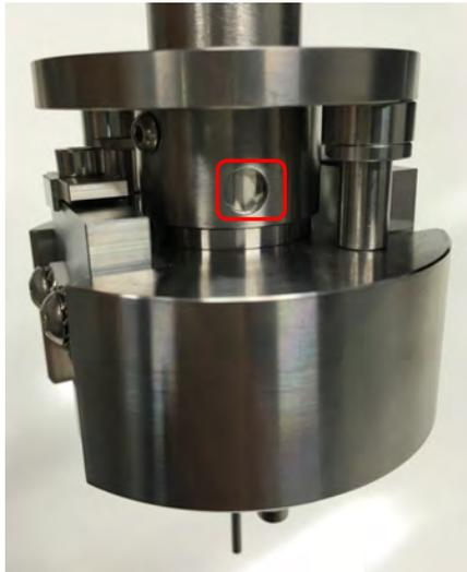
Screw in the rod to hold the e-beam source, align the pins of housing and e-beam source and put the e-beam source into the housing.
