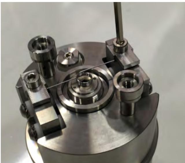
Remove the old filament and slide in a new one. Place the centering rod and tighten the clamping screws. Try to avoid tension in the filament.
