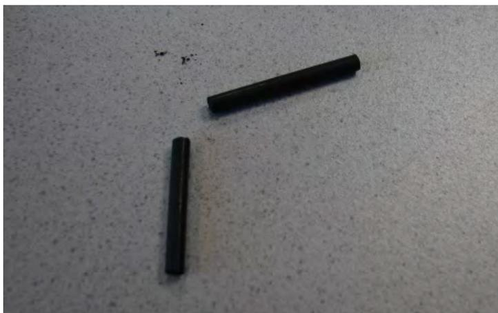
To prepare a carbon platinum rod, take a new 2 mm carbon rod with recess and a platinum inlet.
