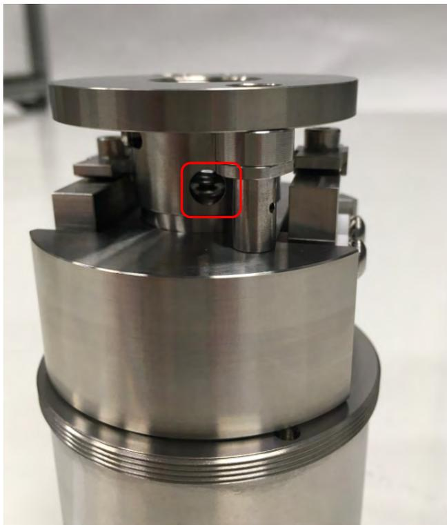
To adjust the rod, turn the collet holder on the bottom of the e-beam source.
