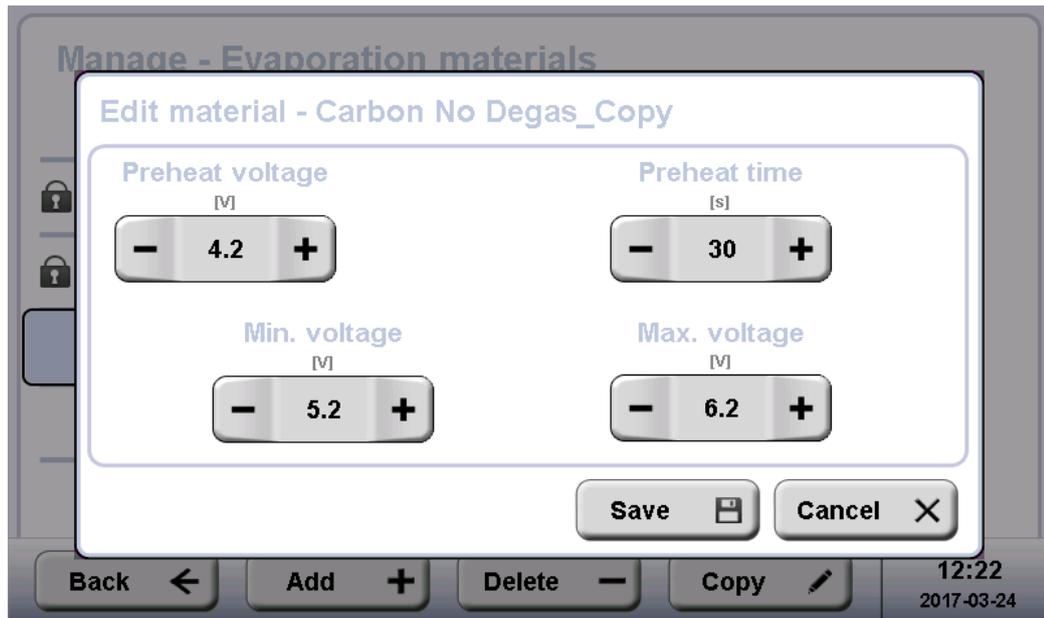
Set a voltage and time for pre-heating the material. The instrument starts with the minimum voltage and ramps up until a suitable deposition rate is reached up to the maximum voltage. Then it controls the parameters to maintain this rate. If a suitable deposition cannot be reached up to the maximum voltage, the deposition is terminated and a message is displayed on the screen.
