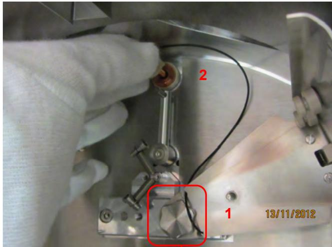
Slide the extra packaged shutter spring (1) on to the pin on the shutter (2).
