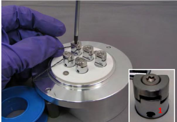
Wind the thread around the other clamps. Take care that the thread slides into the clamping groove (1), follow the path:
