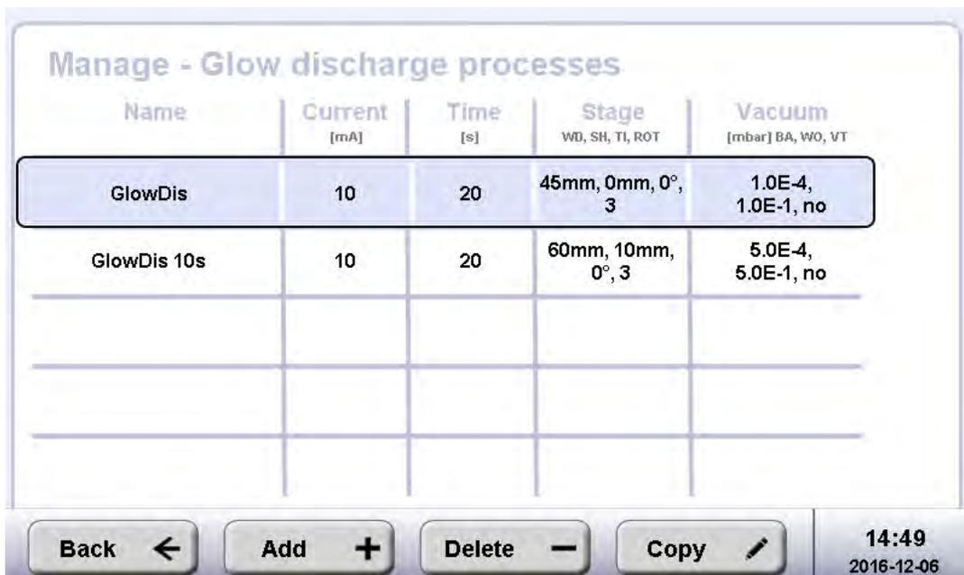
The method defines the current for the glow discharge process and the length of it.
