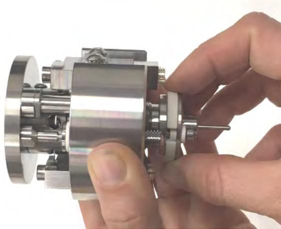
To clean the e-beam source without taking it completely apart, compressed air (oil and water free!) can be used to blow through the hole.
