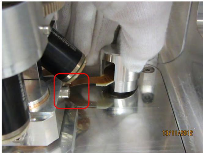
The table is placed on the installed stage. Make sure the pin (1) on the stage and the hole (with O-ring) on the table (2) connect.
