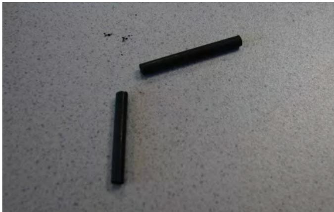
Put one of them back into stock and mount the other one in the copper clamp. Take a new rod and fix it in the holding tool to grind a sharp tip.
