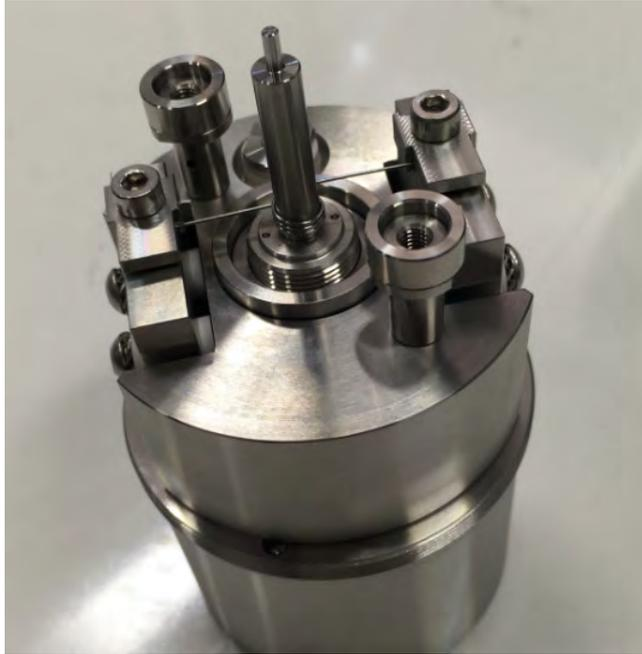
When the tungsten coil is fixed, take out the centering rod. Screw in the collet holder with the carbon rod. Tungsten coil and target are loaded. Make sure the spacers are in place before mounting the aperture.
