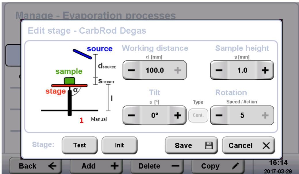
The tilt and height of the stage have to be set manually (see 3.9). The lift height (l) is relative to the surface of the stage.
