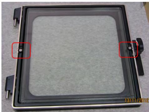
The complete glass can be exchanged by unscrewing both screws on the side to hold the glass. Replace the glass and tighten the screws again.
