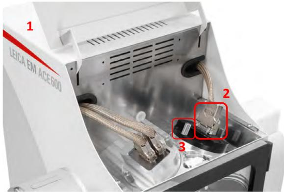
Remove the bayonet ring by turning and insert the sputter target.
