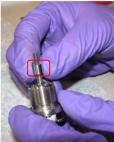
To exchange the tungsten filament loosen the two screws clamping the filament down.
