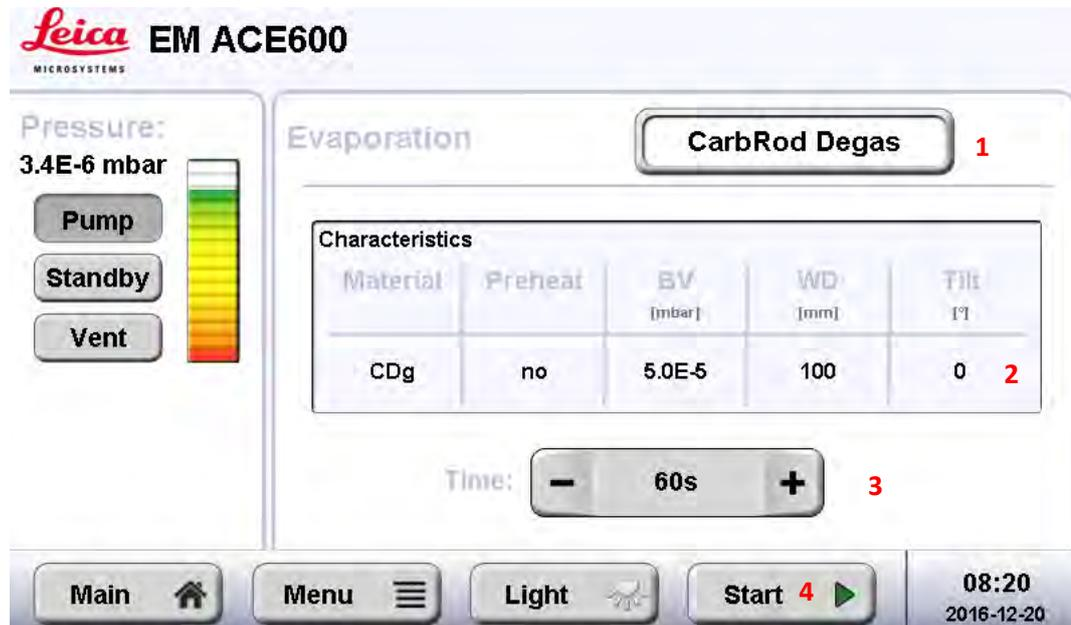
Select a protocol by tapping on it. Once it is marked, by tapping on a specific category, the parameters can be changed. Alternatively, a protocol can be copied and then modified or a new one added.
