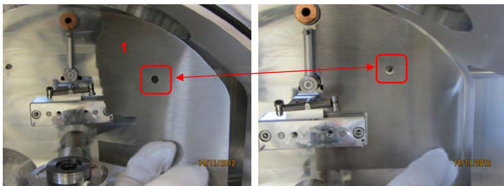
The second shield fits into the top left corner of the chamber wall.
