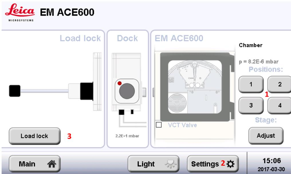
In case the stage must be aligned to transfer the VCT holders push Adjust and align height (1), angle (2) and tilt (3). Set will save the values for the respective position.
