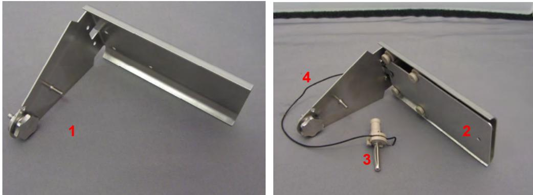
Screw the shutter into the hole (see picture on previous page) in the middle of the rear of the coating chamber by the thumbscrew. Tighten firmly.
