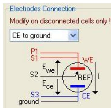
**Fig. 58: CE to Ground connection mode.**
