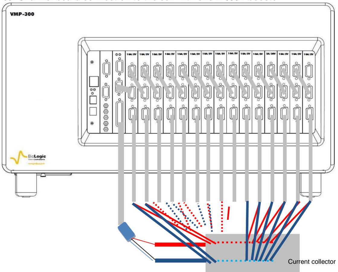
Fig. 64: Channel board connection to the cell with fifteen boosters.
