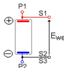
**Fig. 56: Two-electrode connection to a battery cell.**
