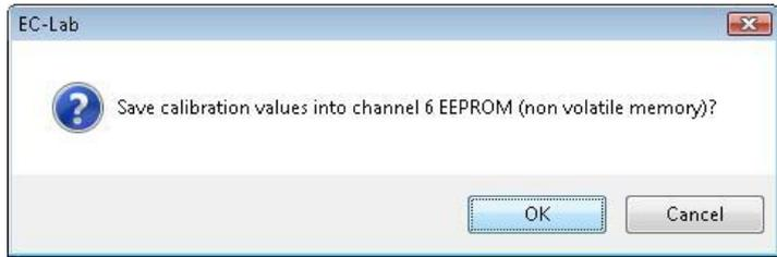
21) If one or more items failed, a warning message indicating that the value of the calibration will not be saved and the calibration process is not completed. Before contacting your local representative, please check again if all the cables were properly connected.
