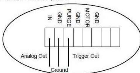
Fig. 72: ALS-RRDE-3A Rotating Disk electrode connection to the cell cable.
