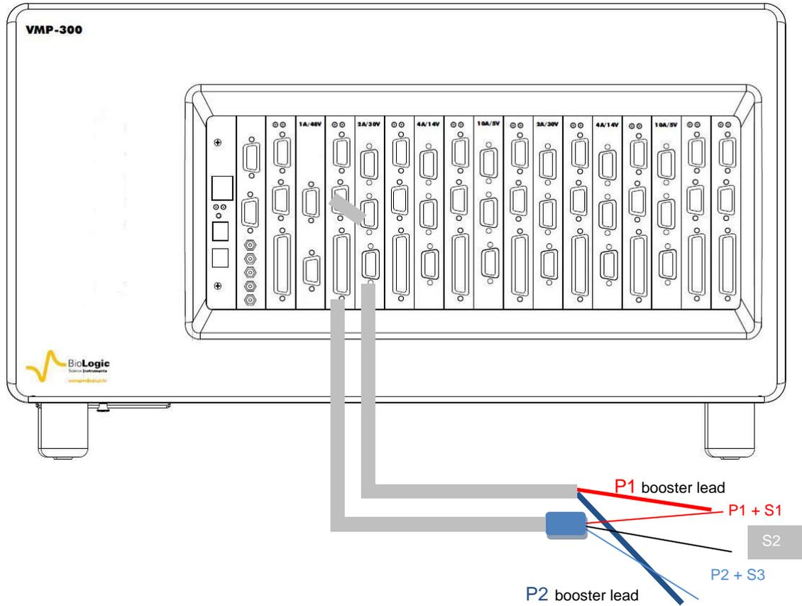
Fig. 63: Channel board connection to the cell with one 2A/30V booster
