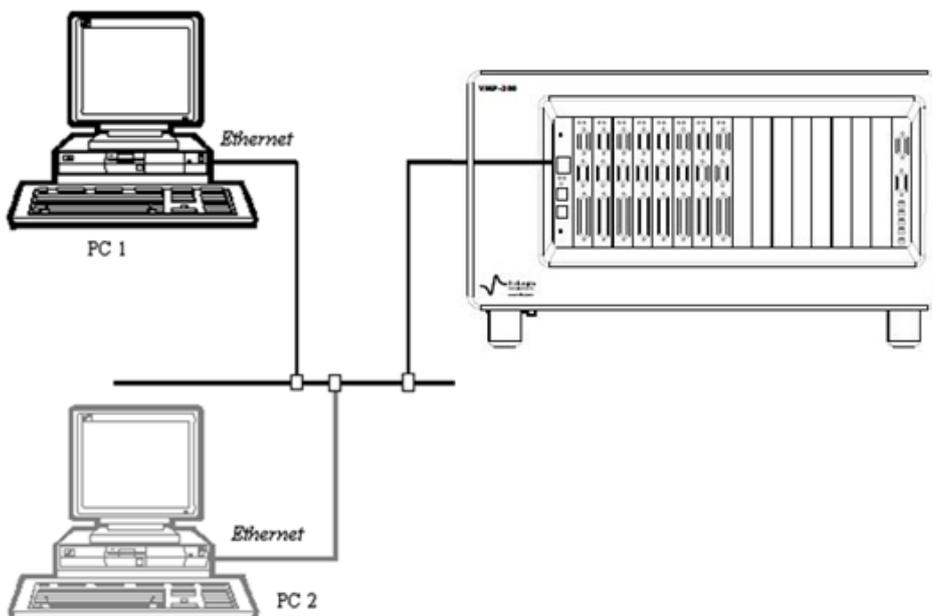
Fig. 26: Ethernet cable for network connection (1 INSTRUMENT, several PCs).
