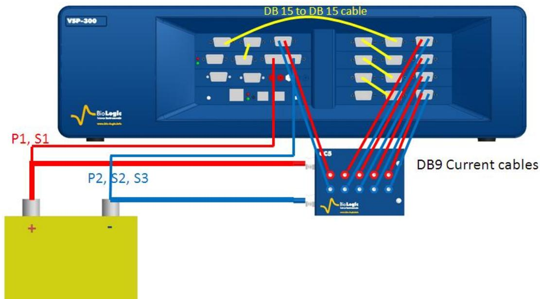
Fig. 82: connection with VSP-300 and CC5 to a battery.
