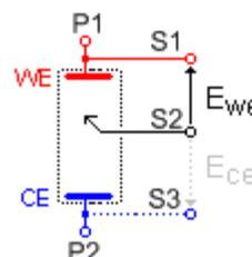
**Fig. 54: Standard three-electrode connection for a classical metal-solution interface.**
