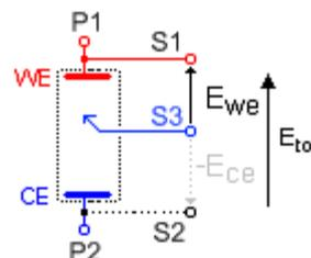
**Fig. 55: Three-electrode connection with a reference electrode.**
