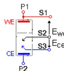
**Fig. 57: Four-electrode connection for a liquid – liquid interface.**
