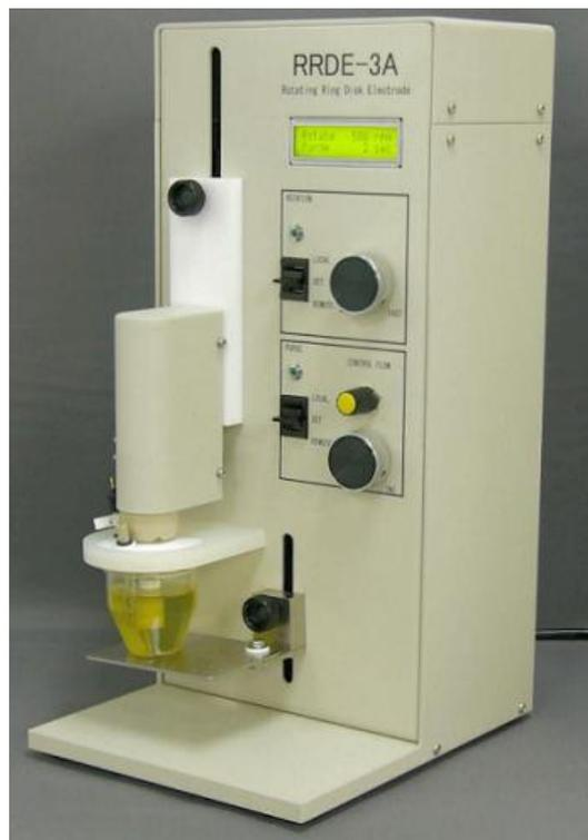
**Fig. 71: ALS-RRDE-3A Rotating Disk electrode**
