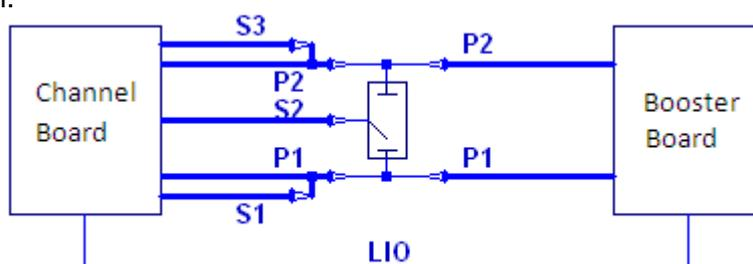
**Fig. 51: Cell connection with 2A, 4A or 10A boosters**
