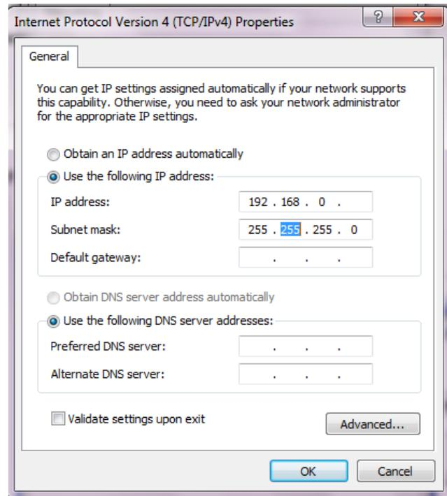
**Fig. 15: TCP/IP properties window.**
