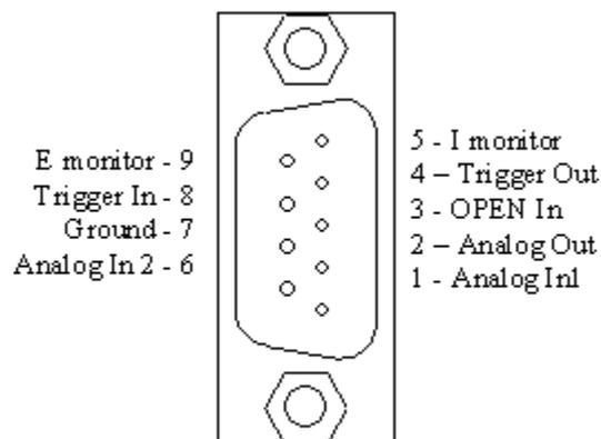
**Fig. 65: Structure of the DB9 connector.**
