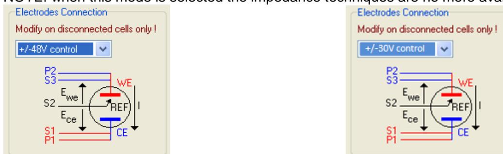
Fig. 60: High voltage control connection mode. Left: +/- 48V for the 1A/48V booster. Right: +/- 30V for the 2A/30V booster.
