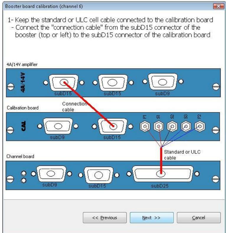
18) Connect the two DB15 connectors of the channel and the amplifier boards as described below and click on the “Next” button.
