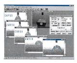
ing of timed interval image capture. Controls motorized syringe and tilting base assembly for advancing and receding contact angle analysis.
