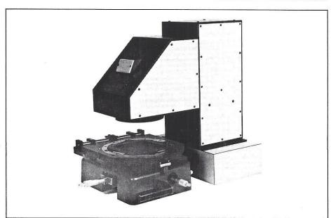
energy transmitted by the secondary mirror is collected by a band-pass tuned photo-feedback detector mounted in the lamp housing and sends that information to the Constant Intensity Controller.
