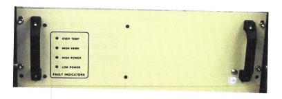
The LED's on the front panel of the unit indicate the operational and error status of the PowerLine L 400.
