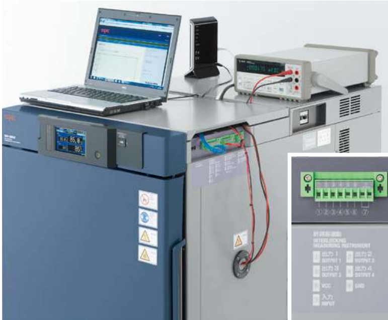
Instrumentation interlock terminals
