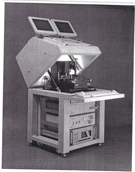
The Integrated Acoustic/Vibration Isolation System allows your Dimension 3100 SPM to produce measurements at the nanometer (lateral) and sub-angstrom (vertical) scales in noisy environments.
