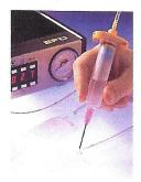
Whether you apply cyanoacrylates or thick sealants, the versatile, easy-to-use 1500XL dispenses absolutely consistent deposits. Unique TEACH function lets the operator establish deposit size, then stores time required for automatic repeat deposits. The dependable 1500XL is trouble-free, with tens of thousands in daily use. For helpful recommendations, call **800-556-3484**.
