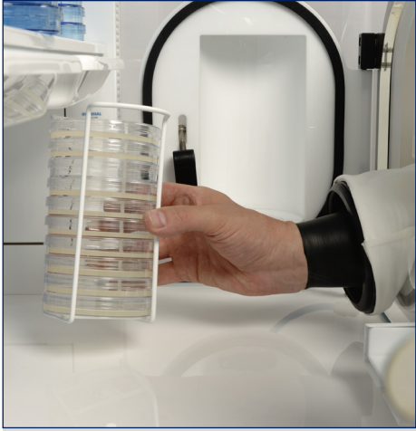
Transfer of plates into a DG250
