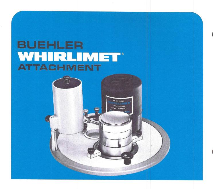
The WHIRLIMET® Attachment is a simple, semi-automatic polishing device that may be adapted to all current and previous BUEHLER 8" (20.3 cm) Polisher/Grinders. An independent motor drives the geared specimen holder at a constant speed in a direction opposite to the wheel rotation. This design prevents directional polishing and ensures a uniform material removal rate.
