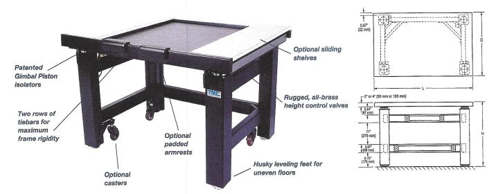
TMC 63-500 Series high-performance lab tables provide an excellent vibration-free working surface for loads up to 350 lbs (160 kg). Now with modular construction, these tables are recommended for use in such diverse applications as: electrophysiology, cell injection, ultramicrotomy, photomicroscopy, scanning tunnel microscopy and confocal laser scanning microscopy.
