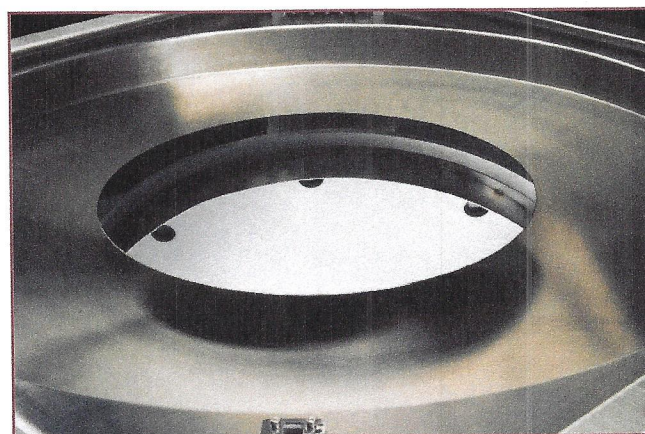
Cee® 300X spin bowl with 300-mm wafer
