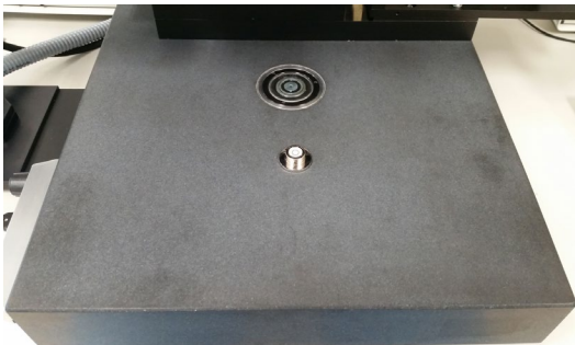
Example: Machine base plate, adjusted with circular level
