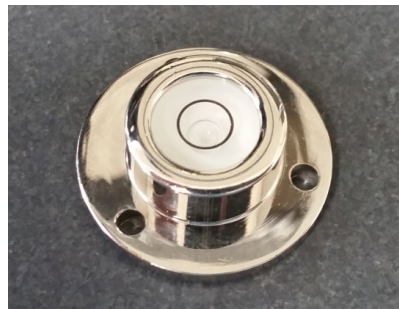
Example: Machine base plate, adjusted with circular level
