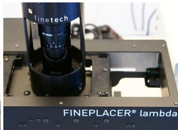
Optics shifting in working position (each position apart from swivel position). Pivot arm cannot be swivelled down.
