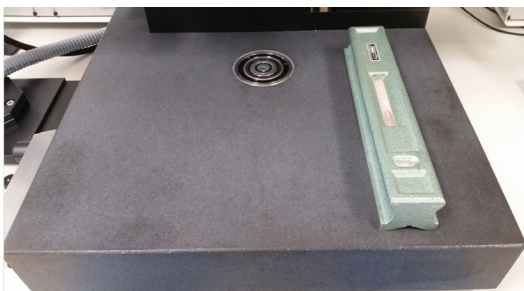
Example: Machine base plate, adjusted with spirit level
